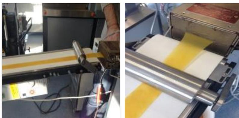
**Figure 43. Pictures demonstrating stretching device attached to extruder to thin the dough sheet achieving thinner intermediates following cutting and drying.**
