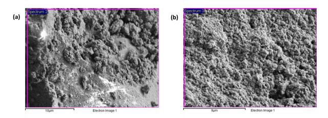
*Figure 6.3: Comparison of surface texture of LDH prepared via (a) conventional, and (b) ultrasonic irradiation routes, at APTES/SDS mole ratio = 5 using ultrasonic horn (UH-LDH5)*
