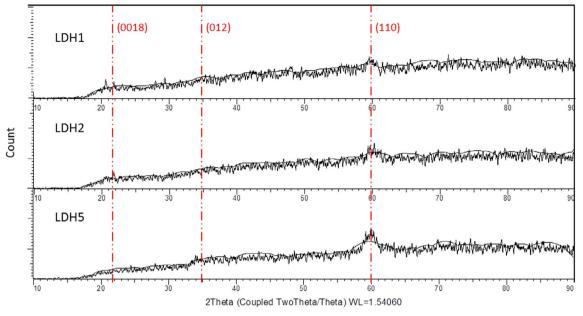
Fig. 4. XRD patterns for LDHn (n = 1, 2 and 5) samples.
