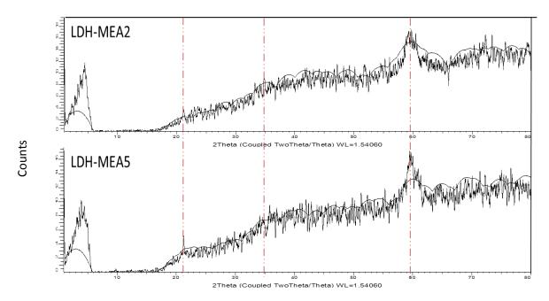
Figure 6.7: XRD patterns for LDH-MEAn (n = 2 and 5) samples
