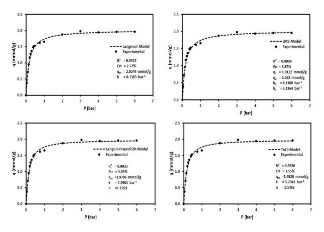
Figure 9.5: Comparison of different isotherm models with experimental data for HPH-14 at temperature of 328 K
