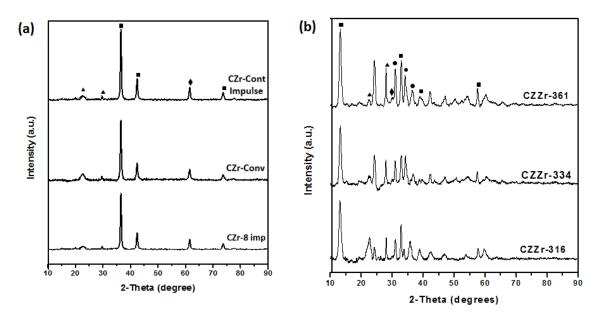
Figure 5.3: XRD pattern for (a) calcined CZr catalysts prepared with variation in ultrasonic impulse at Cu-loading of 30 wt%, and (b) CZZr catalyst prepared with difference in metallic composition. (□) CuO, (○) ZnO, (◊) t-ZrO<sub>2</sub> and (Δ) m- ZrO<sub>2</sub>.
