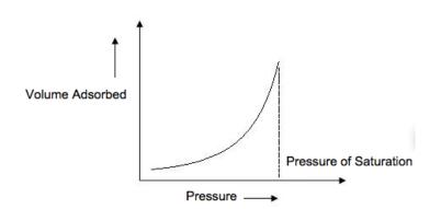
Figure 3.6: Type III adsorption isotherm [12]
