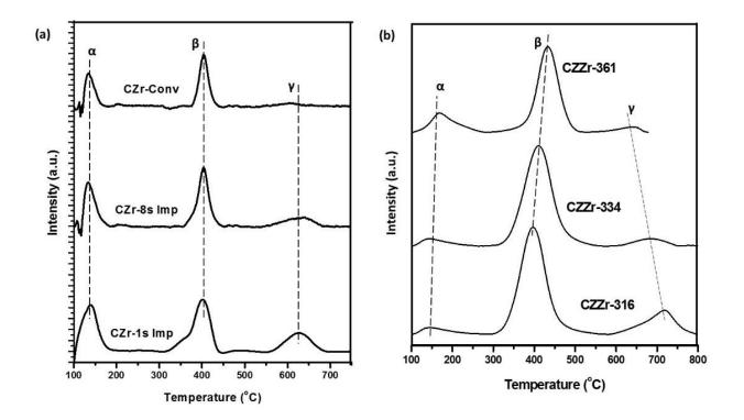
Figure 5.9: CO<sub>2</sub> desorption profile for (a) reduced CZr at various ultrasonic impulse time, and (b) CZZr catalysts at different metal composition
