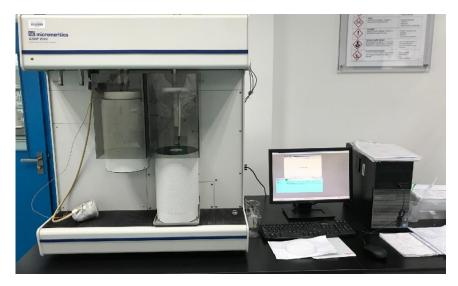
Figure A3.8: Micrometrics ASAP 2020 Surface Area and Porosity Analyser
