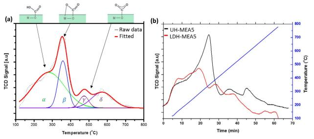
Fig. 16. CO2-TPD of functionalised LDH (a) Deconvolution of the CO2-TPD of UH-MEA5 and (b) Comparison of CO2-TPD of UH-MEA5 and LDH-MEA5.
