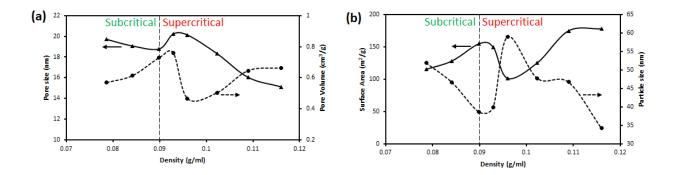
Figure 7.2: BET analysis of prepared LDH with variation in density: (a) variation of pore size and volume, and (b) variation of surface area and particle size
