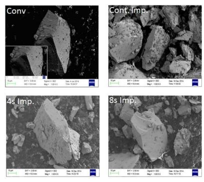
Figure 5.1: SEM Analysis of CZr prepared via Ultrasonic Modulation at different Impulse times (continuous impulse (Cont. Imp.), 4 sec and 8 sec) in comparison with conventional coprecipitation method (Conv)
