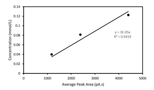
Figure 3.2: GC calibration curve for methanol
