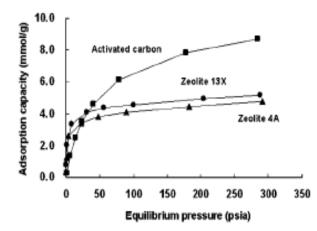
Figure 2.2: Variation of Adsorption Isotherm at High Pressure for Zeolites 13X & 4A and Activated Carbon [20]
