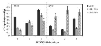
Fig. 11. Comparison of  $CO_2$  uptake by samples prepared via conventional (LDHn) and ultrasonic irradiation route (UH-LDHn and UB-LDHn) at 55 °C and 80 °C.
