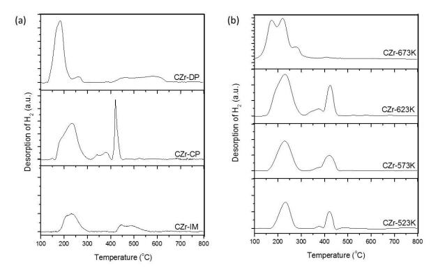
Figure 4.11: H<sub>2</sub>-TPD pattern of (a) CZr catalysts prepared by different method. Catalyst composition: CuO/ZrO<sub>2</sub> = 30/70 (wt.%), (b) CZr catalysts prepared via co-precipitation method at different calcination temperatures compared to CZr catalyst calcined at 673 K (capped phase transformation temperature)
