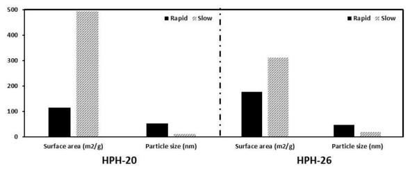
Figure 7.6: Rapid vs slow cooling effect on surface morphology of LDH spheres
