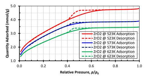
Figure 4.2: BET Isotherm plot of Zirconia support from different calcination temperatures.
