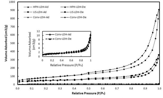
Fig. 5. Nitrogen adsorption-desorption isotherms for Conv-LDH, US-LDH and HPH-LDH samples (inserted image shows the enlarged isotherm for Conv-LDH).
