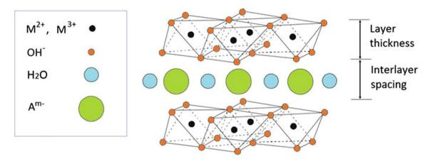
Fig. 1. Structural configuration of layered double hydroxides ([5]-permission obtained).
