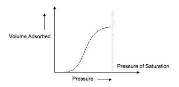
Figure 3.8: Type V adsorption isotherm
