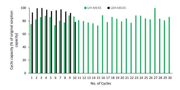
Figure 6.15: TSA Cycles of LDH-MEA5 and UH-MEA5 at 55 °C (30 mins regeneration time at 105 °C in  $N_2$  atmosphere) based on the initial adsorption capacity of 1.45 and 1.37 mmol/g respectively
