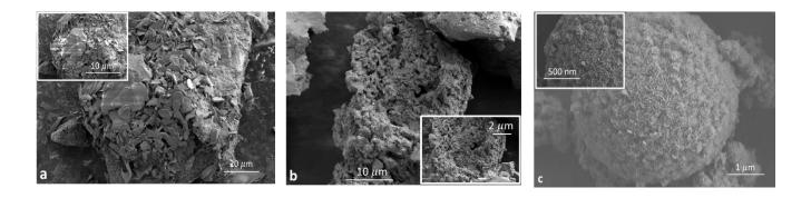
Figure 8.6: SEM images of prepared LDHs (a) Conv-LDH, (b) US-LDH, and (c) HPH-LDH
