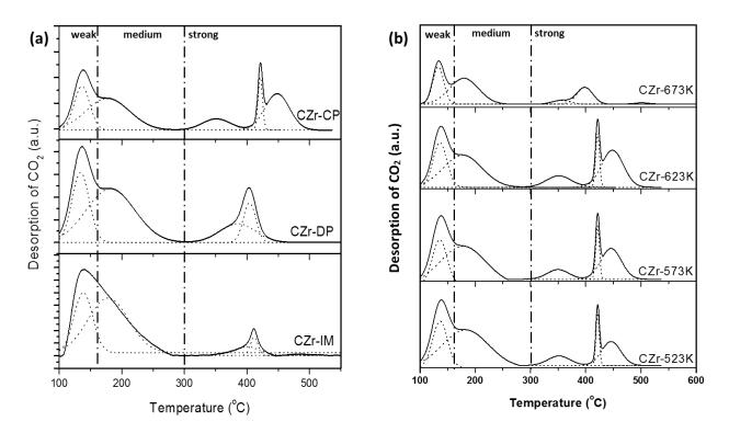
Figure 4.12: CO<sub>2</sub>-TPD pattern of (a) CZr catalysts prepared by different method. Catalyst composition: CuO/ZrO<sub>2</sub> = 30/70 (wt.%), (b) CZr catalysts prepared via co-precipitation method at different calcination temperatures
