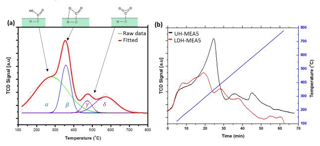
Figure 6.16: CO<sub>2</sub>-TPD of functionalised LDH (a) Deconvolution of the CO<sub>2</sub>-TPD of UH-MEA5 and (b) Comparison of CO<sub>2</sub>-TPD of UH-MEA5 and LDH-MEA5.
