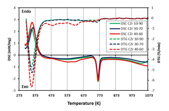
Figure 4.6: Thermal Characterization of IM Catalysts CuO/ZrO<sub>2</sub> at different Cu-loading.
