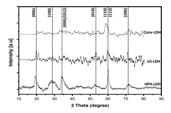
*Figure 8.9: X-ray diffraction patterns of synthesised Mg/Al LDHs via conventional co-precipitation (Conv-LDH), ultrasonic irradiation (US-LDH) and sonochemical-assisted hydrothermal route (HPH-LPH)*
