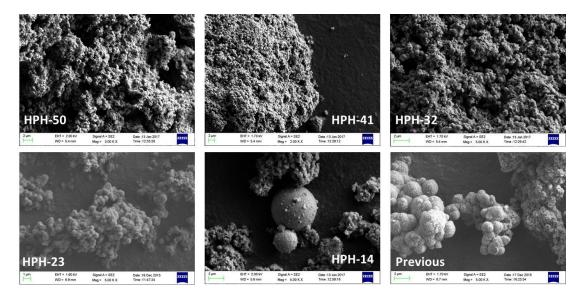
Figure 9.1: SEM images of synthesised CuO/ZnO/ZrO<sub>2</sub> catalyst on Mg-Al LDH support in comparison to previously prepared Mg-Al LDH adsorbent
