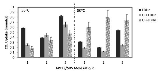
Figure 6.11: Comparison of CO<sub>2</sub> uptake by samples prepared via conventional (LDHn) and ultrasonic irradiation route (UH-LDHn and UB-LDHn) at 55°C and 80°C.
