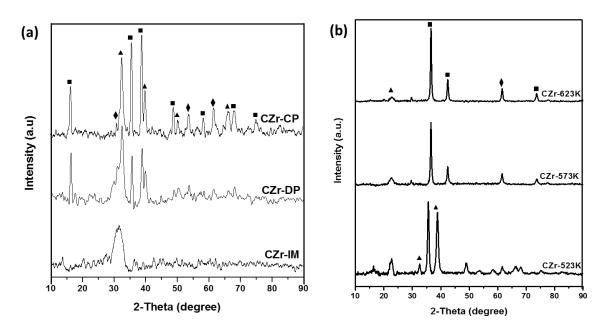
Figure 4.13: XRD pattern of (a) CZr catalysts prepared by different method. Catalyst composition:  $CuO/ZrO_2 = 30/70$  (wt.%), (b) CZr catalysts prepared via co-precipitation method at different calcination temperatures
