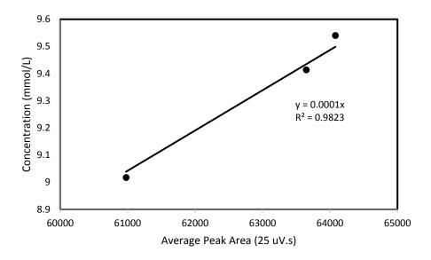
Figure 3.3: GC calibration curve for CO<sub>2</sub>
