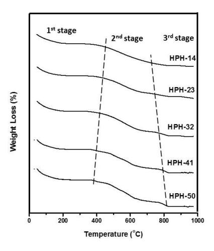
Figure 9.3: Thermogravimetric analysis of composite catalyst
