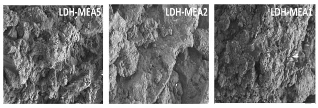
Fig. 2. SEM images of LDH-MEAn at various APTS/SDS mole ratios (n = 5, 2 and 1).
