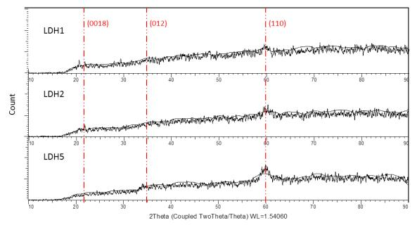
Figure 6.4: XRD patterns for LDHn (n = 1, 2 and 5) samples
