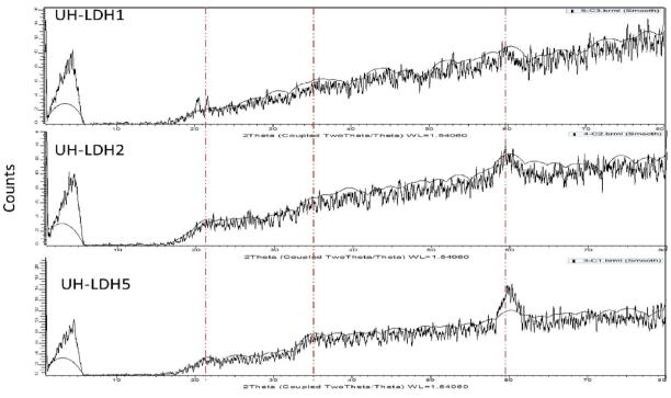
Fig. 6. XRD patterns for UH-LDHn (n = 1, 2 and 5) samples.
