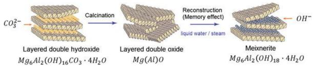
Reaction Scheme 2.1: Reconstruction of thermally activated LDH [89]
