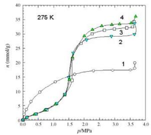
Figure 2.3: Variation of Adsorption Isotherms of CO2 in Coconut Shell-derived Activated Carbon at various Moisture/Dry Carbon Weight Ratios: (1) 0, (2) 1.74, (3) 1.32, (4) 1.65 [41]
