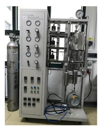
Figure A3.2: Catalyst evaluation/adsorption test rig
