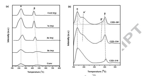
Figure 8: H<sub>2</sub>-TPD profile for (a) reduced CZr at various ultrasonic impulse time, and (b) CZZr catalysts at different metal composition
