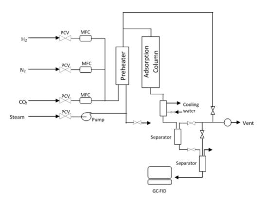
Figure 3.1: Brief schematic diagram of the adsorption column
