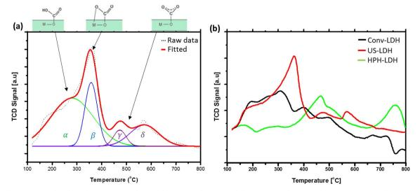
Fig. 8. CO2-TPD of synthesised LDH (a) Deconvolution of the CO2-TPD of UH-LDH and (b) Comparison of CO2-TPD of Conv-LDH, US-LDH and HPH-LDH.
