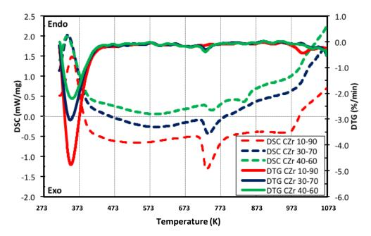
*Figure 4.8: Thermal Characterization of DP Catalysts CuO/ZrO<sub>2</sub> at different Cu-loading.*
