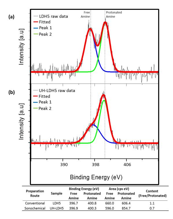
Figure 6.13: N 1s XPS spectra for (a) LDH5 and (b) UH-LDH5
