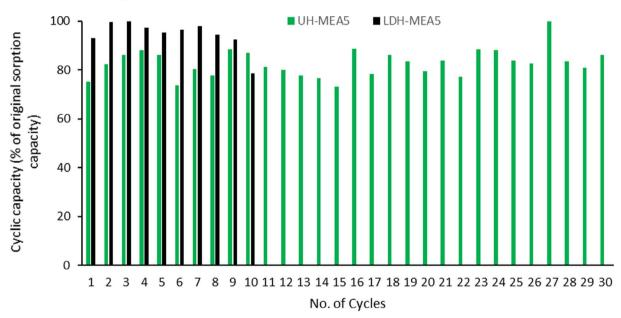
Fig. 15. TSA Cycles of LDH-MEA5 and UH-MEA5 at 55 °C (30 mins regeneration time at 105 °C in N<sub>2</sub> atmosphere) based on the initial adsorption capacity of 1.45 and 1.37 mmol/g respectively.
