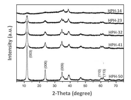
Figure 9.2: XRD pattern synthesised CuO/ZnO/ZrO<sub>2</sub> catalyst on Mg-Al LDH support in comparison to previously prepared Mg-Al LDH adsorbent
