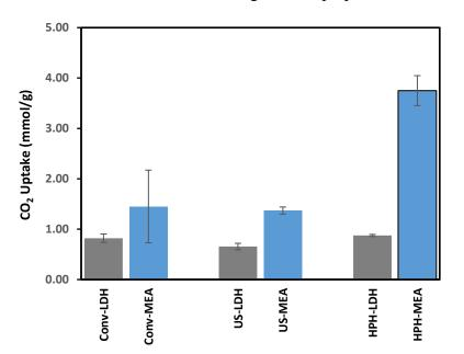
Figure 8.11: Average CO<sub>2</sub> Uptake of LDH and amine-modified LDH prepared via the different routes
