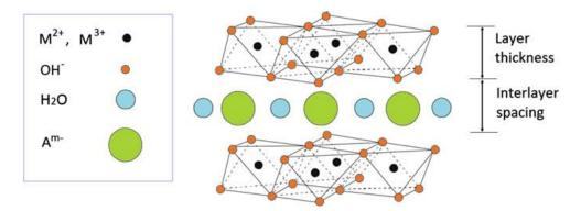
Figure 8.1: Structural configuration of layered double hydroxides [5]
