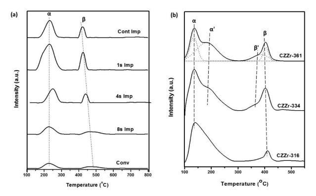
Figure 5.8: H<sub>2</sub>-TPD profile for (a) reduced CZr at various ultrasonic impulse time, and (b) CZZr catalysts at different metal composition
