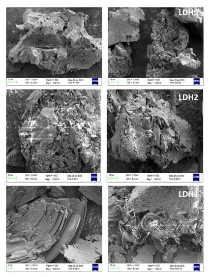
Figure 6.1: SEM Images of prepared LDHs with variation in Surfactant, SDS
