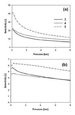
Figure 2.5: Selectivities of CO2 over (a) N2 and (b) CH4 in yCO2= 0.5 mixtures respectively (3 = Zn-DMF (dimethylformamide) coordinated MOF (4,4',4'',4'''-benzene-1,2,4,5tetrayltetrabenzoic acid), 4 = uncoordinated MOF, 5 = highly polar –CF3 coordinated MOF) [51]
