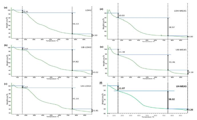
Fig. 14. TGA curves comparing thermal stabilities of LDHs prepared via conventional and ultrasonic irradiation: (a) LDH2, (b) UB-LDH2 and (c) UH-LDH2; as well as with amine modified LDHs: (d) LDH-MEA5 and (e) UB-MEA5 (f) UH-MEA5.
