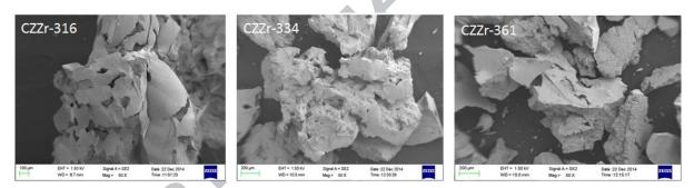
Figure 2: SEM images of prepared CZZr catalysts at varying compositions and continuous impulse ultrasonic irradiation (CZZr-xyz indicates catalyst with  $Cu^{2+}:Zn^{2+}:Zr^{4+}$  molar ratio = x:y:z)
