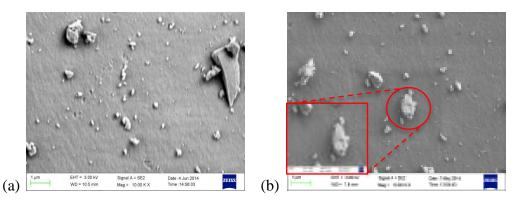
Figure 4.4: SEM image of agglomerated particles on the surface of the Zirconium support at various calcination temperatures: (a) 573K and (b) 623K.
