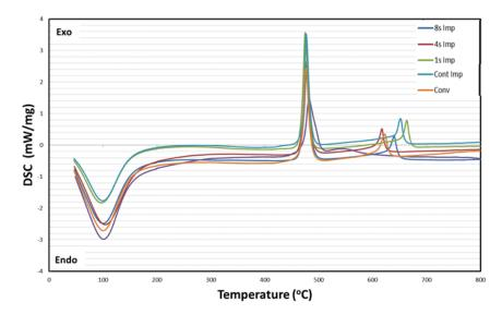
Figure 5.5: DSC profile for CZr catalysts at different ultrasonic impulse
