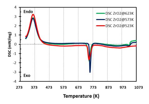
*Figure 4.9: DSC analysis of zirconia support from different calcination temperature.*
