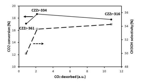
Figure 5.11: Correlation between CO<sub>2</sub>-TPD data with CO<sub>2</sub> conversion and CH<sub>3</sub>OH selectivity for CZZr catalyst
