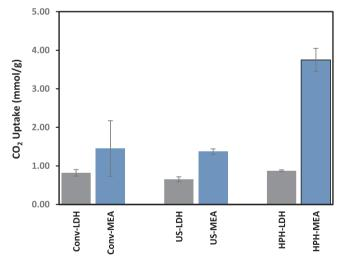
Fig. 11. Average  $CO_2$  Uptake of LDH and a mine-modified LDH prepared via the different routes.
