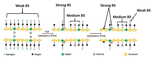
Reaction Scheme 4.4: Proposed decomposition stages for generation of basic sites for calcined CZr catalysts (BS = Basic Sites)
