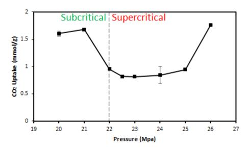
Figure 7.5: Variation of CO<sub>2</sub> uptake with preparation pressure for HPH-M20
