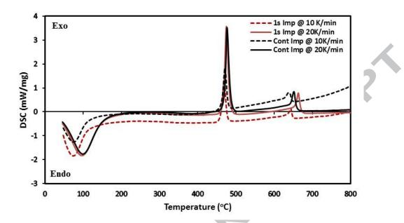
Figure 6: DSC analysis at different heating rate for CZr catalysts prepared with ultrasonic irradiation at 1s and continuous impulse
