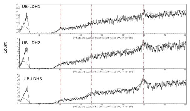
Figure 6.5: XRD patterns for UB-LDHn (n = 1, 2 and 5) samples
