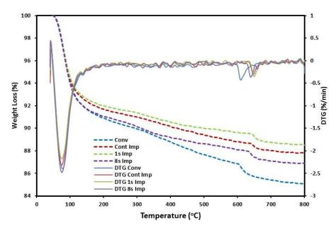
Figure 5.4: TGA-DTA profile for CZr catalysts
