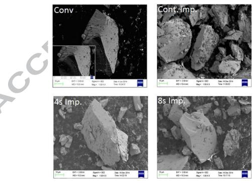
Figure 1: SEM Analysis of CZr prepared via Ultrasonic Modulation at different Impulse times (continuous impulse (Cont. Imp.), 4 sec and 8 sec) in comparison with conventional coprecipitation method (Conv)
