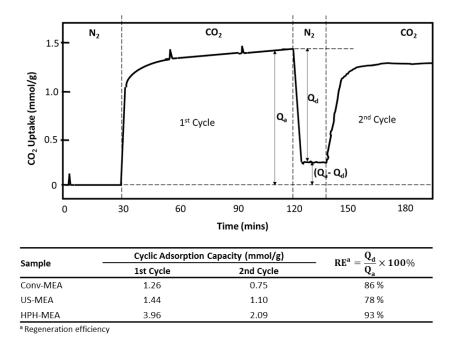
*Figure E8.2: Cyclic adsorption capacity of amine functionalized LDH prepared via different routes*
