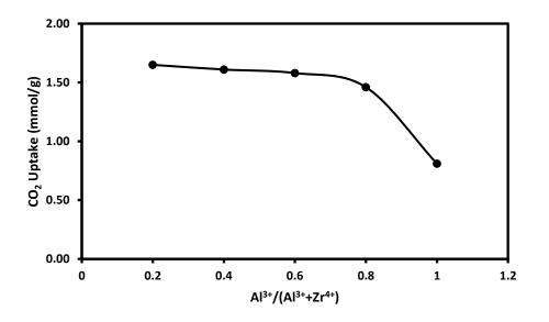
Figure 9.4: Correlation between metal composition and CO<sub>2</sub> uptake for composite catalyst
