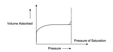
Figure 3.4: Type I adsorption isotherm [12]
