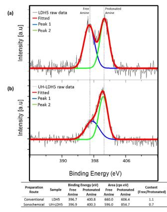
Fig. 13. N 1s XPS spectra for (a) LDH5 and (b) UH-LDH5.
