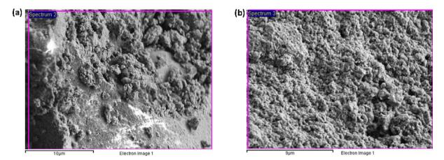
Fig. 3. Comparison of surface texture of LDH prepared via (a) conventional, and (b) ultrasonic irradiation routes, at APTS/SDS mole ratio = 5 using ultrasonic horn (UH-LDH5).
