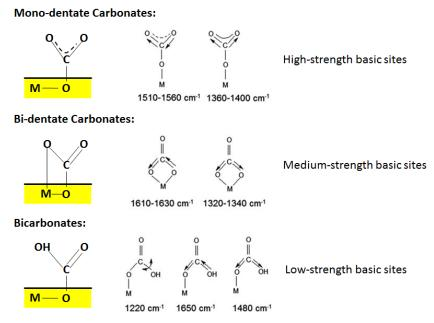
Figure 8.2: Infrared bands of adsorbed CO<sub>2</sub> on LDH surface [9]
