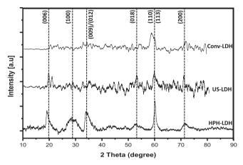
Fig. 9. X-ray diffraction patterns of synthesised Mg/Al LDHs via conventional co-precipitation (Conv-LDH), ultrasonic irradiation (US-LDH) and sonochemical-assisted hydrothermal route (HPH-LPH).
