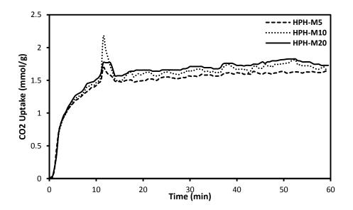
Figure 7.5: CO<sub>2</sub> uptake of amine modified HPH-26 at varying amine loading of 5g, 10g and 20g
