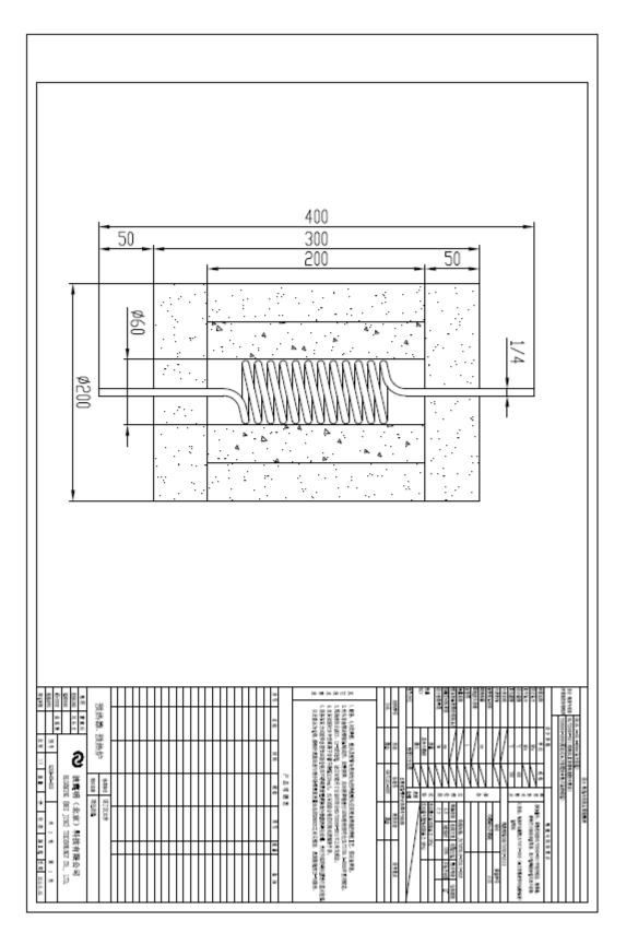
Figure A3.5: Design sheet for the preheater
