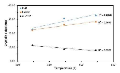
Figure 4.14: Variation of crystallite sizes of CuO, t-ZrO<sub>2</sub> and m-ZrO<sub>2</sub> with calcination temperature
