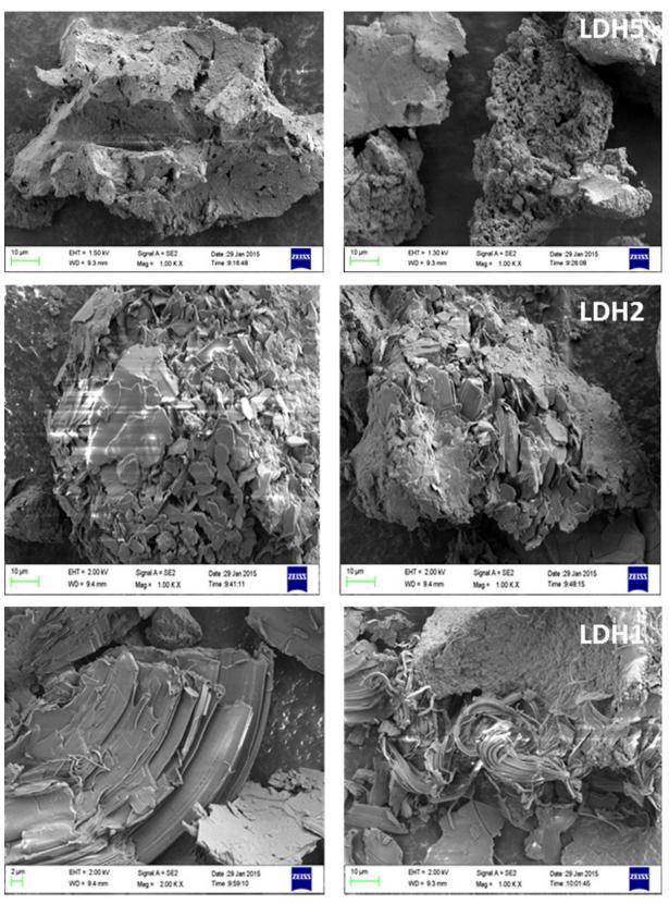
Fig. 1. SEM Images of prepared LDHs with variation in Surfactant, SDS.
