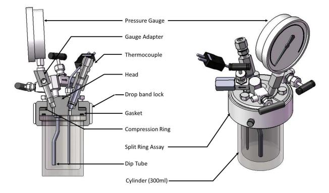
Figure 7.1: Schematic diagram of the hydrothermal reactor
