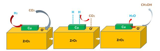
Figure 2.9: Hydrogen spill-over mechanism in  $CO_2$  hydrogenation for methanol synthesis using  $Cu/ZrO_2$  catalyst
