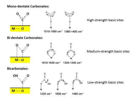
Figure 2.8: Infrared bands of adsorbed CO<sub>2</sub> on LDH surface [97]
