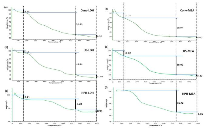
Fig. 10. TGA curves comparing thermal stabilities of LDHs prepared via conventional and ultrasonic irradiation: (a) Conv-LDH, (b) UH-LDH and (c) HPH-LDH; as well as with amine modified LDHs: (d) Conv-MEA (e) UH-MEA and (f) HPH-MEA.
