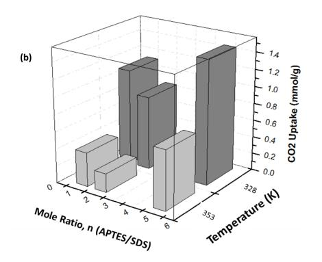
Figure 6.10: CO<sub>2</sub> Uptake for (a) LDHn and (b) LDH-MEAn (with n being the molar ratio of APTES to SDS)
