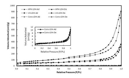
Figure 8.5: Nitrogen adsorption-desorption isotherms for Conv-LDH, US-LDH and HPH-LDH samples (inserted image shows the enlarged isotherm for Conv-LDH)
