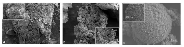
Fig. 6. SEM images of prepared LDHs (a) Conv-LDH, (b) US-LDH, and (c) HPH-LDH.
