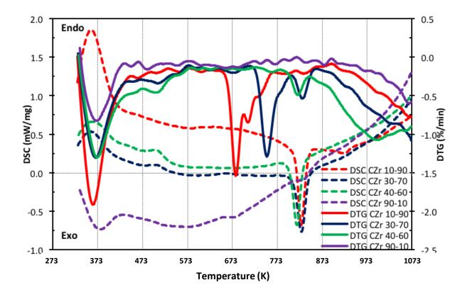
*Figure 4.7: Thermal Characterization of CP Catalysts CuO/ZrO<sub>2</sub> at different Cu-loading.*
