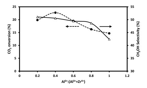
Figure 9.6: Correlation between CO<sub>2</sub> conversion and methanol selectivity with metal composition
