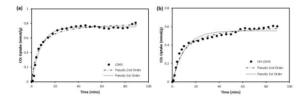
Figure 6.17: Comparison of kinetic models with experimental results for CO<sub>2</sub> uptake on (a) LDH5 and (b) UH-LDH5
