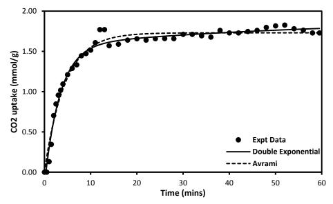
Figure 7.8: Simulation of adsorption kinetics based on experimental data of HPH-M20
