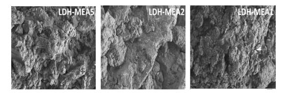
Figure 6.2: SEM images of LDH-MEAn at various APTES/SDS mole ratios (n = 5, 2 and 1)
