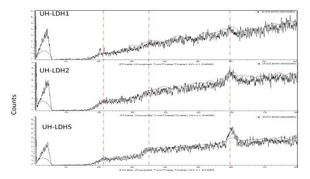
Figure 6.6: XRD patterns for UH-LDHn (n = 1, 2 and 5) samples
