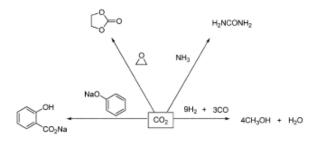
Reaction Scheme 1.2: CO<sub>2</sub> Utilization [2]
