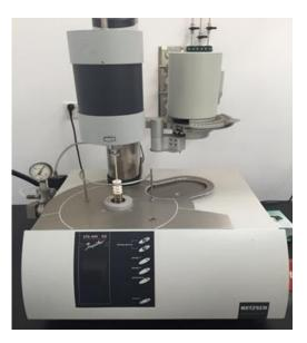
Figure A3.1: Thermogravimetric Analyser
