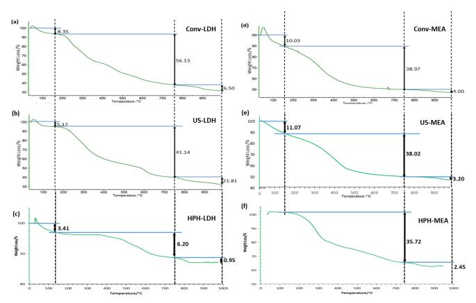
Figure 8.10: TGA curves comparing thermal stabilities of LDHs prepared via conventional and ultrasonic irradiation: (a) Conv-LDH, (b) UH-LDH and (c) HPH-LDH; as well as with amine modified LDHs: (d) Conv-MEA (e) UH-MEA and (f) HPH-MEA
