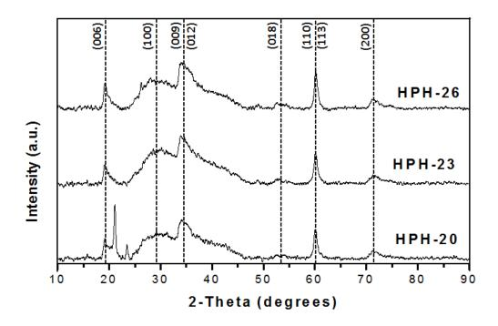
Figure 7.4: X-ray spectra for synthesised LDH nano-spheres prepared at various pressures at a temperature of 723 K
