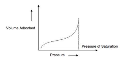
Figure 3.5: Type II adsorption isotherm [12]
