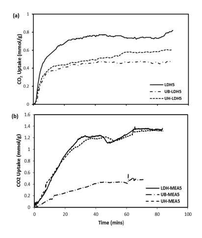
Figure 6.12: Comparison of CO<sub>2</sub> uptake by samples prepared via conventional (LDHn) and ultrasonic irradiation route (ultrasonic horn, UH-LDHn and ultrasonic bath, UB-LDHn) with APTES/SDS mole ratio, n = 5 at 55°C (a) prior MEA extraction, and (b) post MEA extraction
