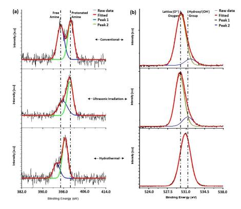
*Figure 8.7:* XPS spectra of conventionally-, ultrasonically- and hydrothermally-prepared LDHs for (a) N 1s and (b) O 1s
