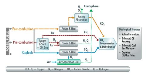
Figure 1.2: Summarized flow sheet for various CCS technology
