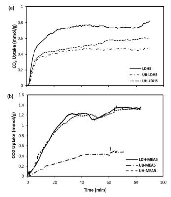
**Fig. 12.** Comparison of CO<sub>2</sub> uptake by samples prepared via conventional (LDHn) and ultrasonic irradiation route (ultrasonic horn, UH-LDHn and ultrasonic bath, UB-LDHn) with APTS/SDS mole ratio, n = 5 at 55 °C (a) prior MEA extraction, and (b) post MEA extraction.
