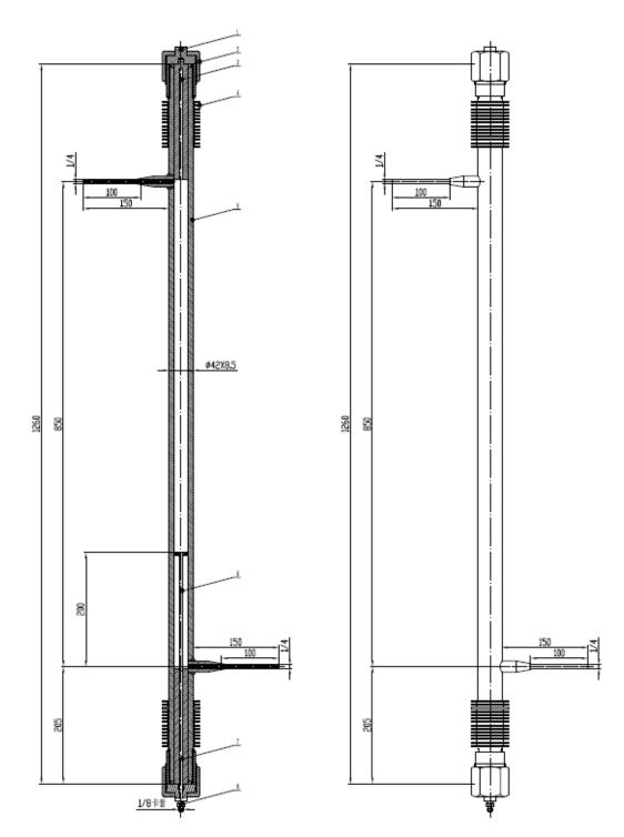
Figure A3.3: Design specification for the adsorption column (dimensions are in mm)
