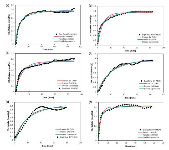
Fig. 12. Comparison of different kinetic models with experimental data generated for adsorption kinetics of CO<sub>2</sub> on (a) Conv-LDH, (b) US-LDH, (c) HPH-LDH, (d) Conv-MEA, (e) US-MEA and (f) HPH-MEA under and 55 °C and 1 atm.
