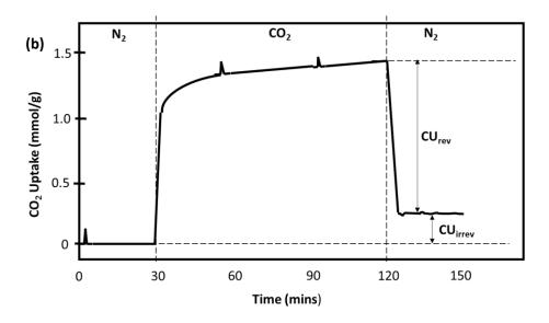
Figure 6.9: Example of (a) TGA curve for CO<sub>2</sub> adsorption, (b) recoverable CO<sub>2</sub> uptake using TSA at 105 °C in  $N_2$  atmosphere.
