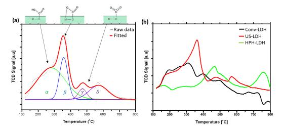
*Figure 8.8*: CO<sub>2</sub>-TPD of synthesised LDH (a) Deconvolution of the CO<sub>2</sub>-TPD of UH-LDH and (b) Comparison of CO<sub>2</sub>-TPD of Conv-LDH, US-LDH and HPH-LDH.
