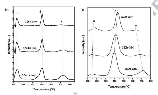
Figure 9: CO<sub>2</sub> desorption profile for (a) reduced CZr at various ultrasonic impulse time, and (b) CZZr catalysts at different metal composition
