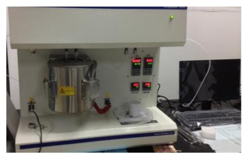
Figure A3.9: Temperature-Programmed Desorption (TPD) reactor
