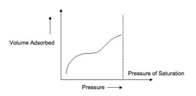
Figure 3.7: Type IV adsorption isotherm [12]
