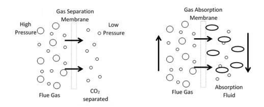
Figure 1.3: Absorption mechanism for gas separation and gas absorption membrane
