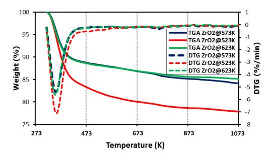
Figure 4.5: TG-DTG analysis of zirconia support from different calcination temperature.
