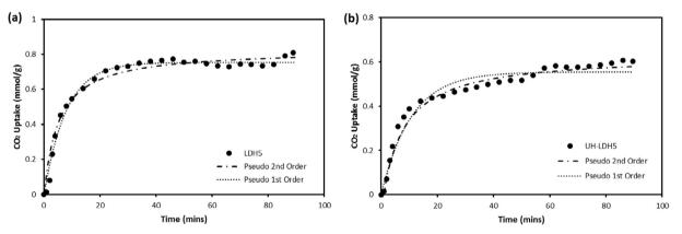
Fig. 17. Comparison of kinetic models with experimental results for CO<sub>2</sub> uptake on (a) LDH5 and (b) UH-LDH5.
