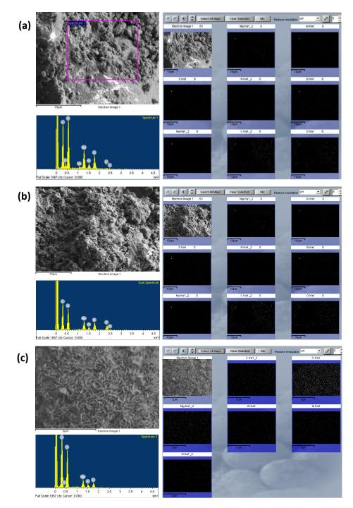
Figure E8.1: EDX elemental dispersion across the internal micro structures of the prepared adsorbents: (a) Conv-LDH, (b) US-LDH and (c) HPH-LDH
