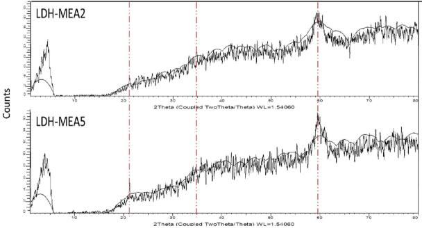
Fig. 7. XRD patterns for LDH-MEAn (n = 2 and 5) samples.
