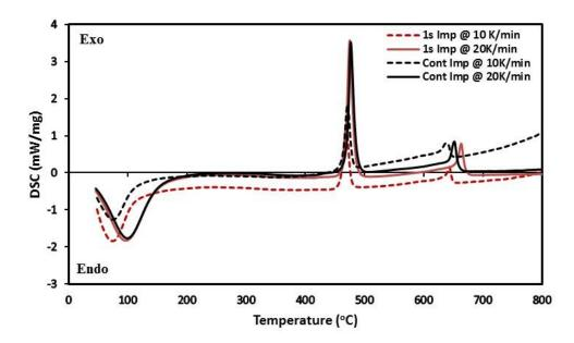
Figure 5.6: DSC analysis at different heating rate for CZr catalysts prepared with ultrasonic irradiation at 1s and continuous impulse
