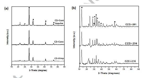
Figure 3: XRD pattern for (a) calcined CZr catalysts prepared with variation in ultrasonic impulse at Cu-loading of 30 wt%, and (b) CZZr catalyst prepared with difference in metallic composition. ( $\Box$ ) CuO, ( $\circ$ ) ZnO, ( $\diamond$ ) t-ZrO<sub>2</sub> and ( $\Delta$ ) m- ZrO<sub>2</sub>
