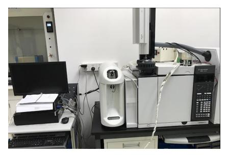
Figure A3.6: Gas Chromatograph-flame ionization detector (GC-FID)
