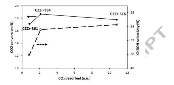
Figure 11: Correlation between CO<sub>2</sub>-TPD data with CO<sub>2</sub> conversion and CH<sub>3</sub>OH selectivity for CZZr catalyst
