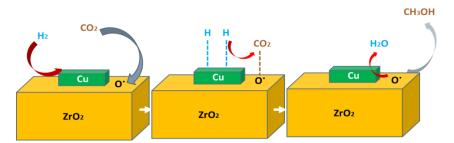
*Figure 4.1: Hydrogen spill-over mechanism in CO2 hydrogenation for methanol synthesis using Cu/ZrO<sub>2</sub> catalyst.*
