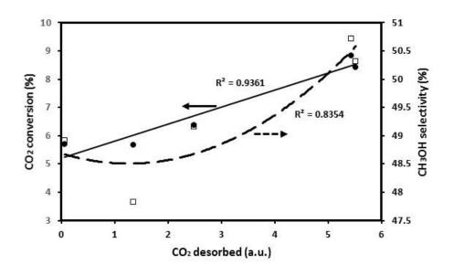
Figure 5.10: Correlation between CO<sub>2</sub>-TPD data with CO<sub>2</sub> conversion and CH<sub>3</sub>OH selectivity for CZr catalyst
