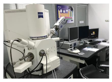
Figure A3.7: Scanning Electron Microscopy (SEM) – Energy Dispersive X-ray Spectroscopy (EDX)
