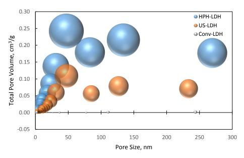
*Figure 8.4: Total pore volume of various pore sizes of Conv-, US- and HPH-LDH samples (bubble size indicates relative amount of pore size)*
