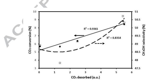
Figure 10: Correlation between CO<sub>2</sub>-TPD data with CO<sub>2</sub> conversion and CH<sub>3</sub>OH selectivity for CZr catalyst
