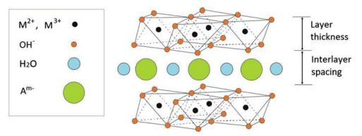
Figure 2.7: Structural configuration of layered double hydroxides [58]
