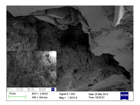
Figure C4.1: SEM image of zirconia aerogel, calcined at 523K.
