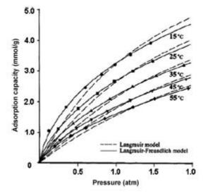
Figure 2.1: Variation of adsorption isotherm with temperature for activated carbon [38]
