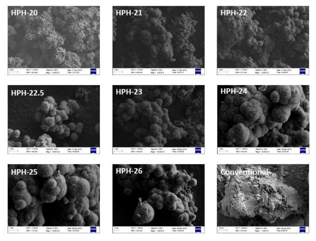
*Figure 7.3: SEM images of Mg-Al LDH nano-spheres prepared at various pressures, 20-26 MPa in comparison to conventionally prepared LDH*
