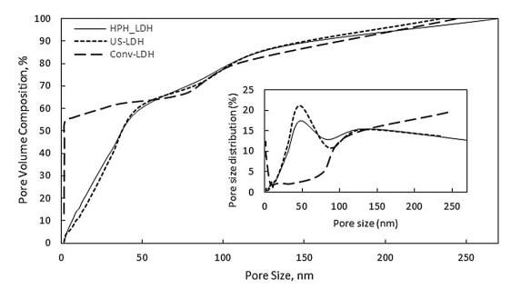
Fig. 3. Pore size distribution of Conv-, US- and HPH-LDH samples.
