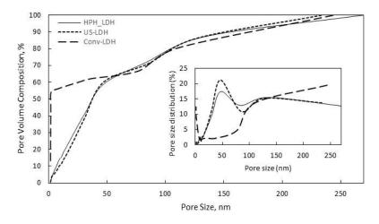
Figure 8.3: Pore size distribution of Conv-, US- and HPH-LDH samples
