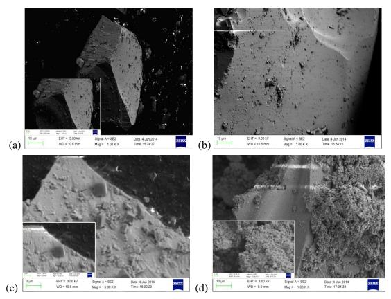
Figure 4.3: SEM image of the surface of the ZrO2 support doped with Cu at calcination temperatures of 623K prepared via (a) undoped ZrO2 support, (b) IM method, (c) CP method and (d) DP method.
