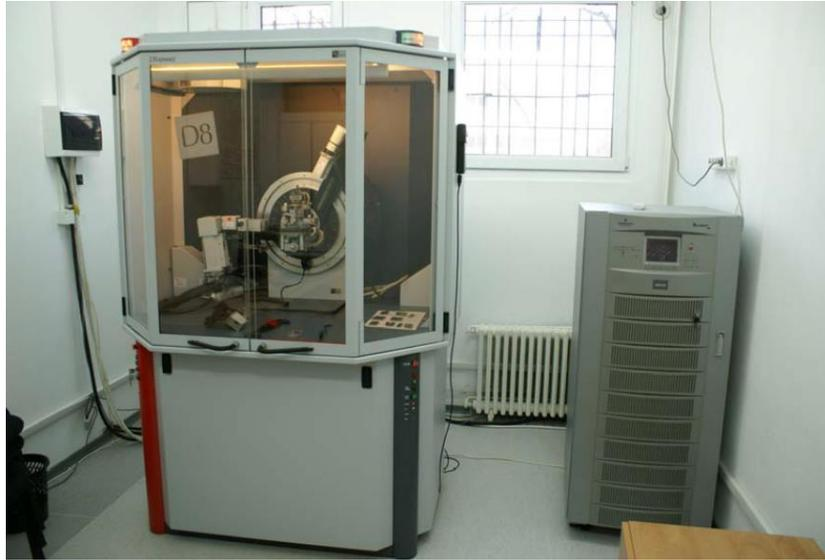
Figure 4-8: X-ray Diffractometer of Bruker
