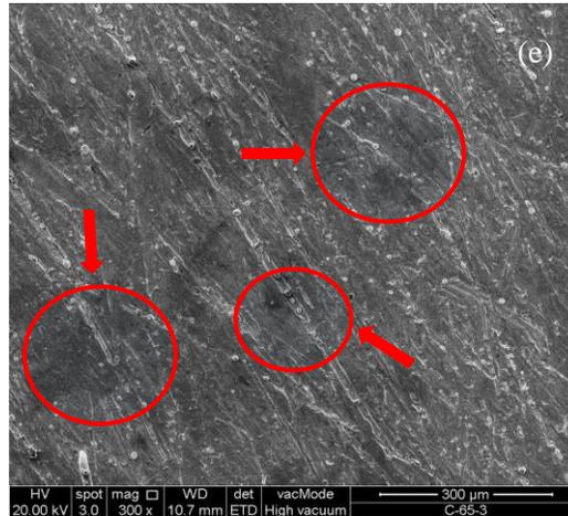
**Figure 5-23:** Shows SEM analysis of corrosion test on copper strip. **Figure 5-23** (a) is morphology of bare copper strip and (b), (c), (d) and (e) are SEM images of copper strips after corrosion test in base salt, molten salt dispersed 0.01, 0.05 and 0.1 wt. %, respectively.
