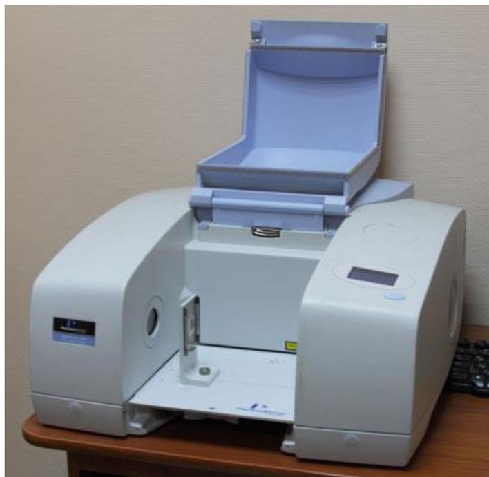
**Figure 4-7:** FTIR instrument of Perkin Elmer
