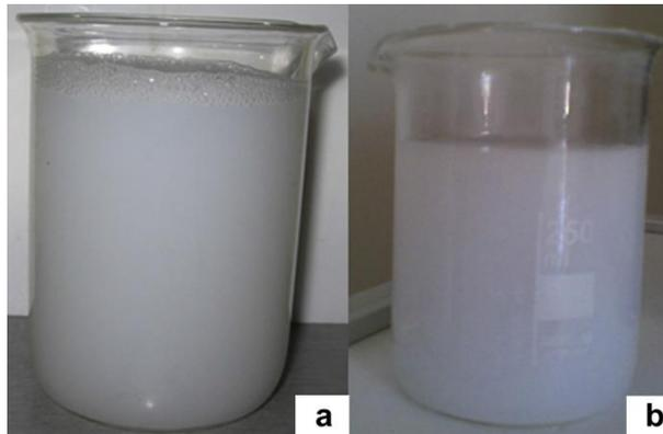
**Figure 2-16:** Photograph of Al<sub>2</sub>O<sub>3</sub> nanofluid (a) with triton X-100 surfactant and (b) without triton X-100 surfactant [140].
