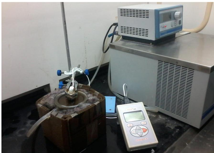
**Figure 4-4:** Thermal conductivity setup
