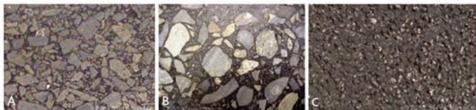
Figure 2-1 Different asphalt pavement surfaces: A) Dense-Graded HMA; B) SMA; C) Open-Graded HMA (Tom and Krishna Rao, 2007)
