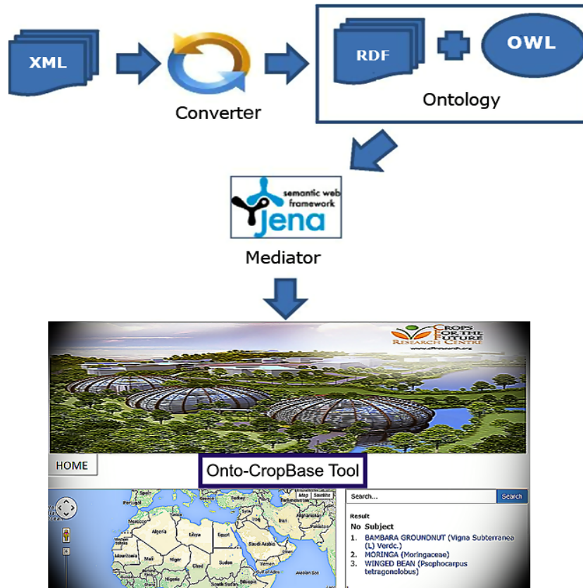
Figure 3.9: Onto-CropBase architecture showing the tool's components
