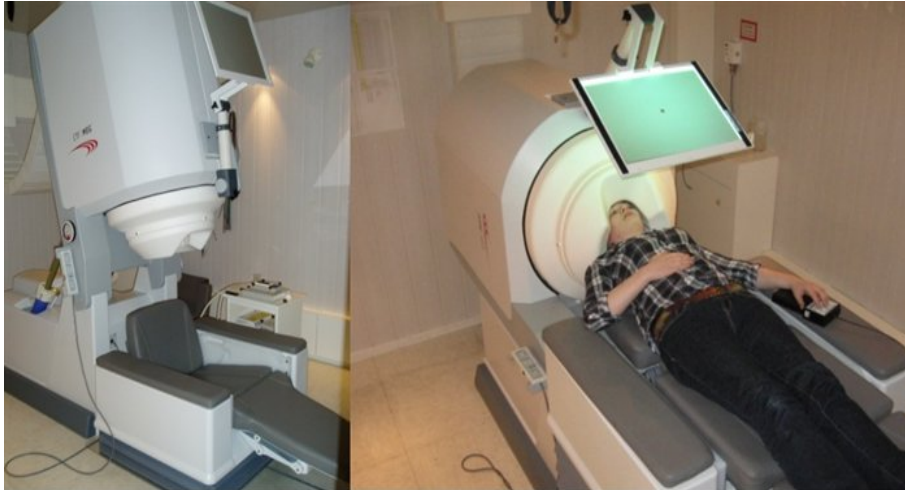
Figure 1: MEG scanner at Sir Peter Mansfield Magnetic Imaging Centre (SP-MMIC), University of Nottingham. Patient undergoing an experiment, scanner can be used in horizontal or vertical position. Source: https://www.nottingham.ac.uk/magres/facilities/meg.aspx
