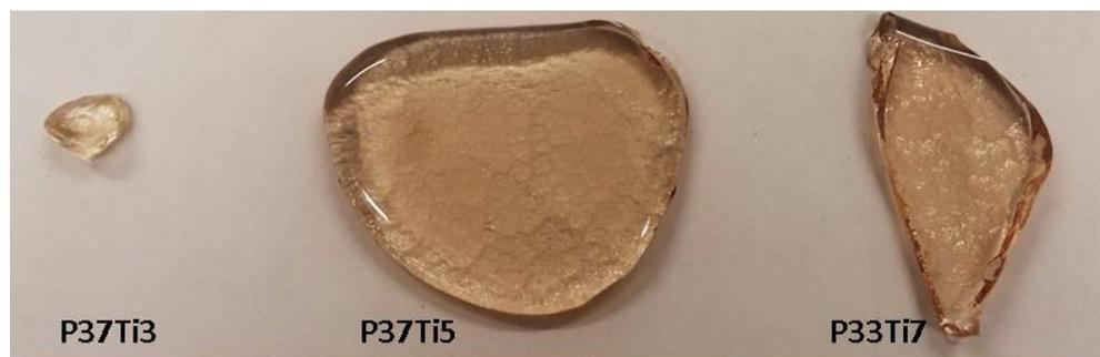
**Figure 5.3:** Representative image showing the effect of increasing Ti content on glass colour.
