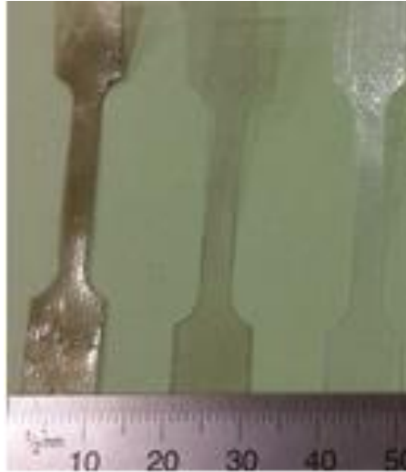
Figure 3.4: Representative image of the dog bone shape polymer films tested
