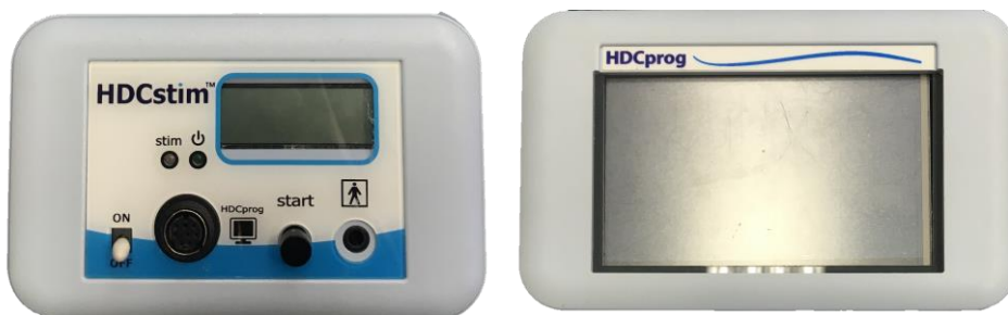
Figure 4-1: HDCstim (left) and touch screen HDCprog (right). tDCS machine provided by Newronika.
