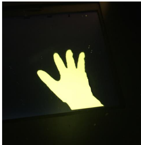
Figure 5-3: ‘4-digit’ hand in which the little finger is no longer visible. This happened as soon as the hand entered MIRAGE due to the glove being worn.
