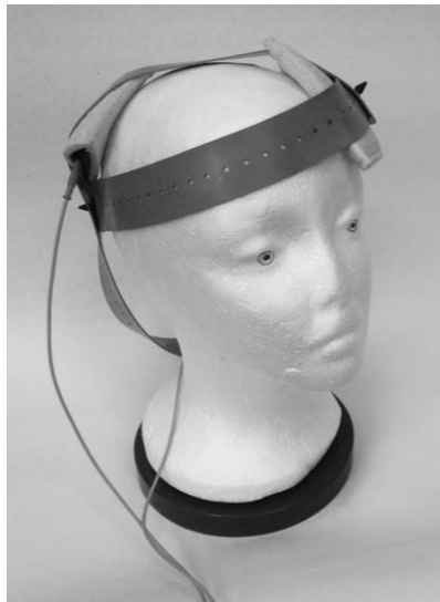
Figure 4-2: Electrode montage placement. In this example secured with bands so the electrodes are visible. For actual testing a cap was used.
