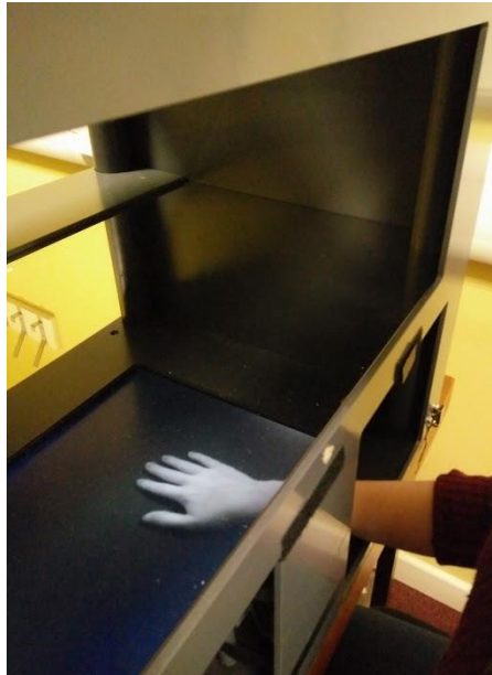
Figure 2-2: Image of the MIRAGE showing participant placing right hand inside. Virtual hand is viewable in its veridical location through the mirror.
