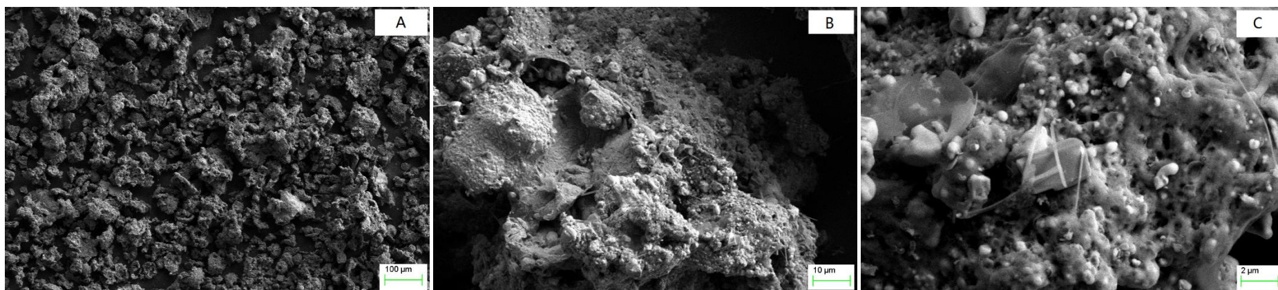
Figure 7-3 SEM images of char pyrolyzed from dunaliella in CO 2 at 400 °C with magnification of A x 100, B x 1000, C x 5000; at 550 °C, D x 100, E x 1000, F x 5000; at 700 °C, G x 100, H x 1000, I x 5000
