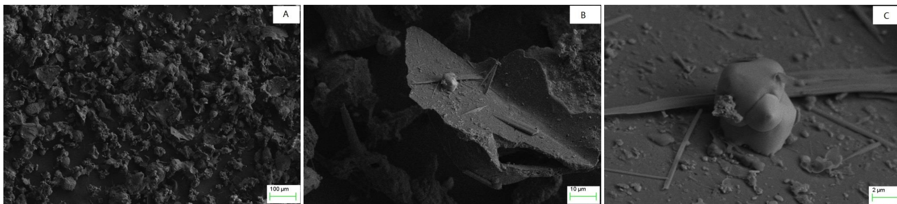
Figure 6-2 SEM images of char pyrolyzed from spirulina at 400 °C with magnification of A x 100, B x 1000, C x 5000; at 550 °C, D x 100, E x 1000, F x 5000; at 700 °C, G x 100, H x 1000, I x 5000
