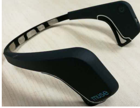
Figure 5.1: The Muse EEG headset used in this study.
