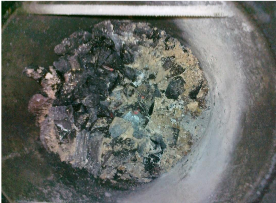
Figure 6-11: Biochar bed as an unsuccessful attempt in tar capture.
