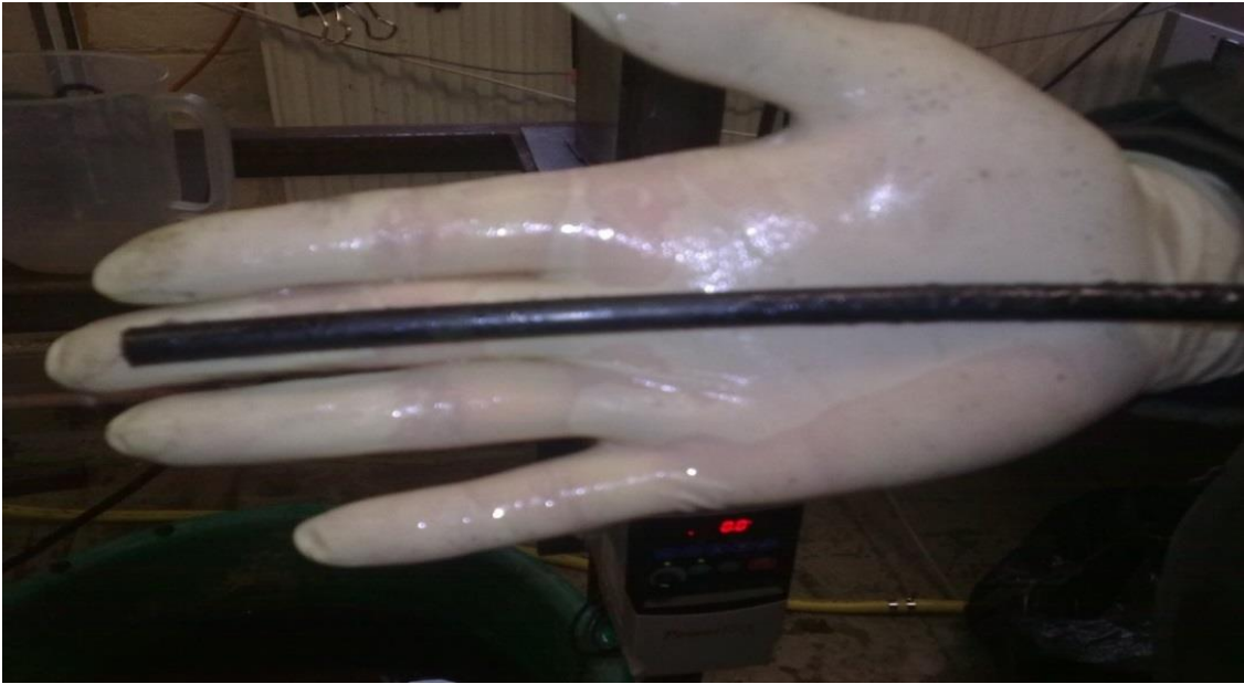
Figure 6-1: Tar in spray water drainage pipe.
