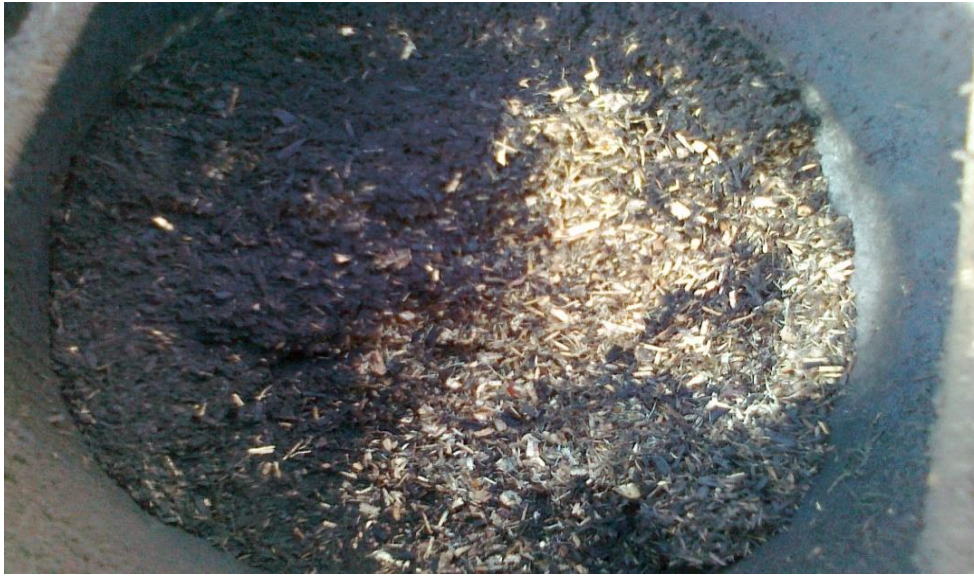
Figure 6-7: Image of tar trapped by small woodchips (3-10 mm).
