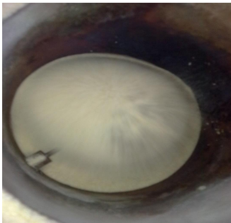
Figure 3-11: Air bubble rising in the reactor.
