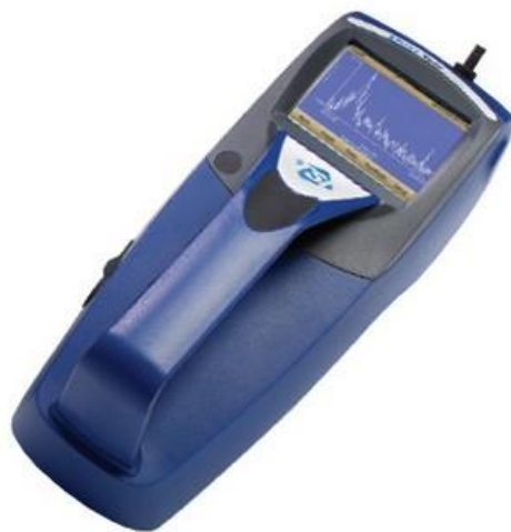
Figure 3-13: TSI DustTrak used to measure the concentration of dust particles
