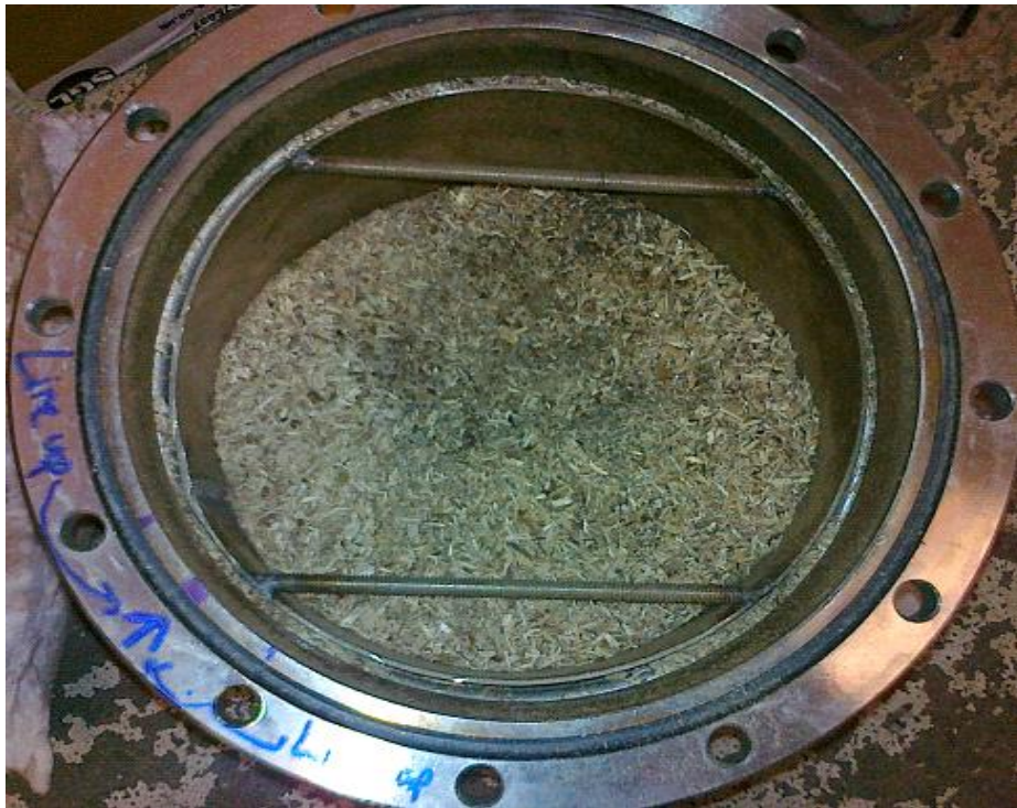
Figure 6-6: Small wood chips (3-10 mm) bed for tar arrest experiment.
