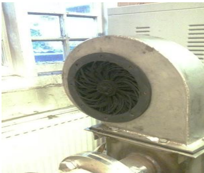
Figure 5-2: Mop fan installed in mop fan unit.
