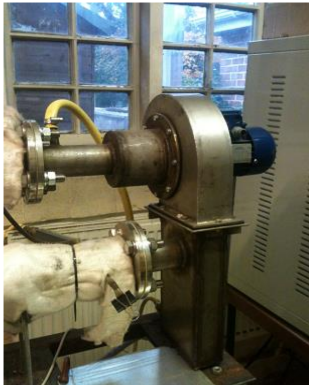
Figure 5-1: Mop fan unit installed on the gasifier.
