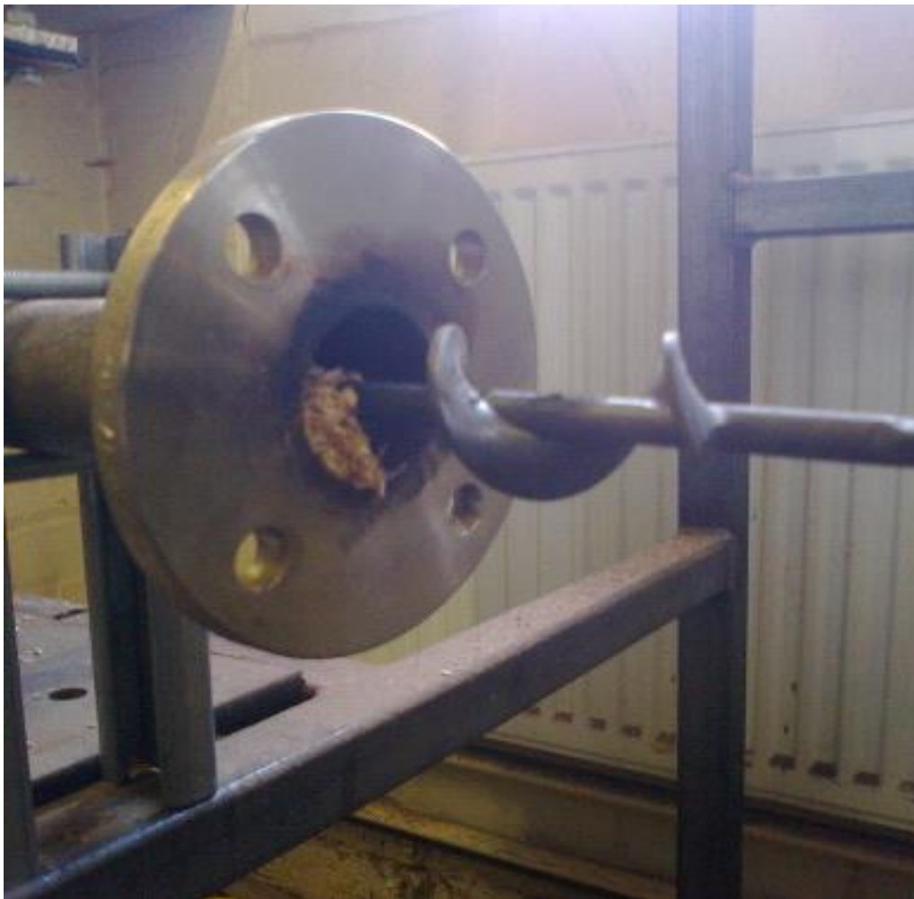
Figure 3-5: Auger feeding wood chips to the gasification reactor from the feeder hopper.
