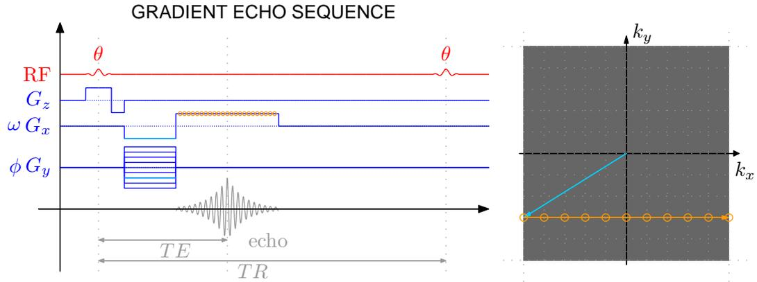
**Figure 2.2.4:** Timing diagram of a gradient echo (GE) sequence: RF pulse (red), gradients (blue) and echo signal (grey), with marked echo time (TE) and repetition time (TR) (left). Gradients positions marked in light blue correspond to the movement in k-space plotted in the same colour and signal sampling trajectory is indicated by orange circles (right).
