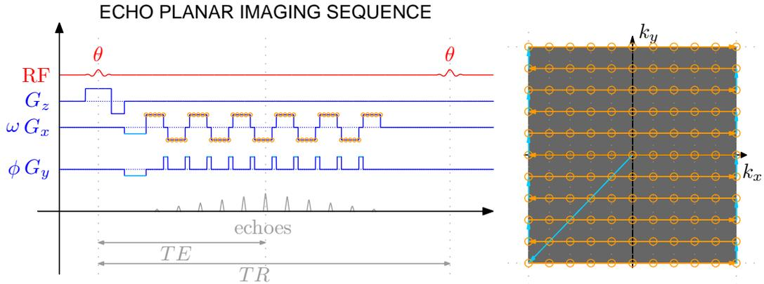
**Figure 2.2.7:** Timing diagram of an echo planar imaging (EPI) sequence: RF pulse (red), gradients (blue) and echo signal (grey), with marked echo time ( $TE$ ) and repetition time ( $TR$ ) (left). Gradients positions marked in light blue correspond to the movement in k-space plotted in the same colour and signal sampling trajectory is indicated by orange circles (right).
