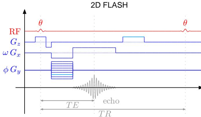
**Figure 2.3.1:** Timing diagram of a 2D FLASH sequence: RF pulse (red), gradients (blue) with their current positions (light blue) and echo signal (grey), with marked echo time (TE) and repetition time (TR).
