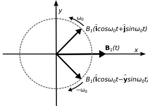
**Figure 2.1.5:** The two components of the magnetic field,  $\mathbf{B}_1$ , rotating in the clockwise and anti-clockwise directions.
