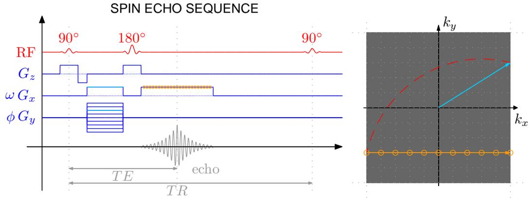
**Figure 2.2.3:** Timing diagram of a spin echo (SE) sequence: RF pulses (red), gradients (blue) and echo signal (grey), with marked echo time (TE) and repetition time (TR) (left). Gradients positions marked in light blue correspond to the movement in k-space plotted in the same colour. The effect of the refocusing pulse is plotted in red and signal sampling trajectory is indicated by orange circles (right).
