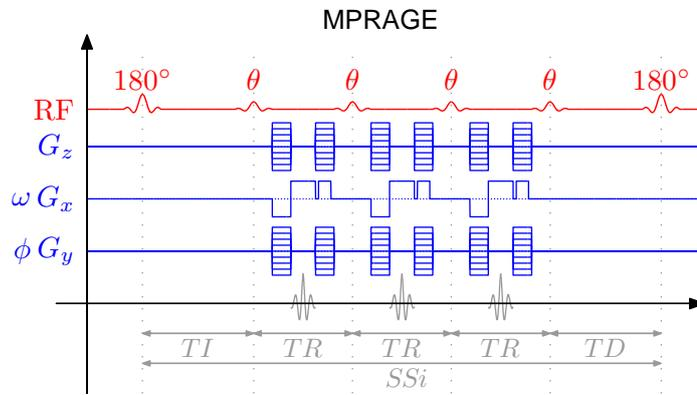
**Figure 2.3.2:** Timing diagram of a 3D MPRAGE sequence: RF pulse (red), gradients (blue) with their current positions (light blue) and echo signal (grey), with marked echo time (TE) and repetition time (TR); time points a-d are used in the equations for  $T_1$  mapping in the next section.
