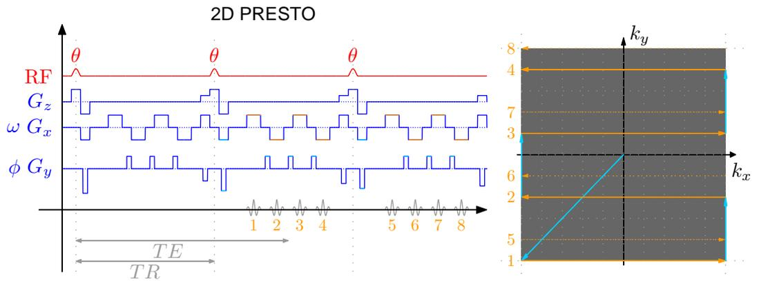
**Figure 2.3.6:** Timing diagram of the 2D PRESTO sequence: RF pulse (red), gradients (blue) and echo signal (grey), with marked echo time ( $TE$ ) and repetition time ( $TR$ ) (left). Gradients positions marked in light blue correspond to the movement in k-space plotted in the same colour and signal sampling trajectory is indicated by orange circles (right).
