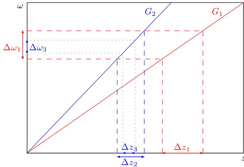
**Figure 2.2.1:** Plot illustrating the relation between bandwidth, gradient strength and slice thickness. The bandwidth  $\Delta\omega_1$  gives a thinner slice  $\Delta z_2 < \Delta z_1$  using the stronger gradient  $G_2$ , but the narrower bandwidth  $\Delta\omega_3 < \Delta\omega_1$  gives a thinner slice  $\Delta z_3 < \Delta z_2$  with the same gradient.
