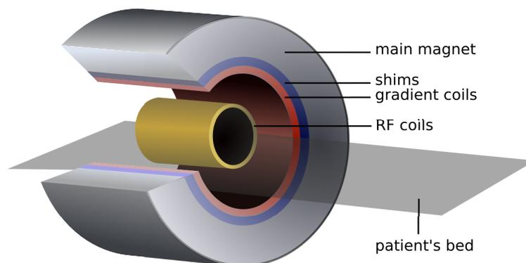
**Figure 2.2.8:** Schematic illustration of the MR scanner architecture.
