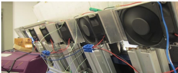
Fig. 7. 15 Integration of TEG-fan-heat-sink waste heat recovery system with heat pipe-based PV collector
