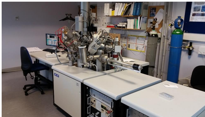
Figure 2.5. (Top Left) Schematic of primary ions hitting a surface and releasing secondary ions (Top Right) ©IONTOF schematic of a SIMS instrument. (Bottom) Image of the ToF-SIMS IV instrument.
