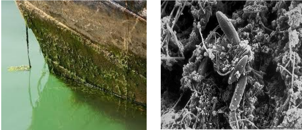
Figure 1.1. (Left) Image of a fouled ship hull on the macroscale. (Right) Scanning electron micrograph image of a developed biofilm on a steel surface after 8-weeks immersion in an industrial water cooling system. [8]
