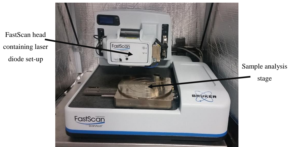
Figure 2.3. (Top) Schematic of the basic set-up of an atomic force microscope. The movement of the tip across the surface is detected by a laser deflected onto the top of the cantilever. (Bottom) Photograph of the Bruker Icon FastScan AFM.
