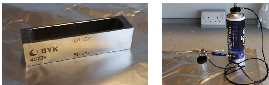
Figure 2.2. (Left) Image of BYK paint applicator for applying coatings to glass slides (Right) Badger airbrush used to apply coating to SEM stubs and glass coverslips.
