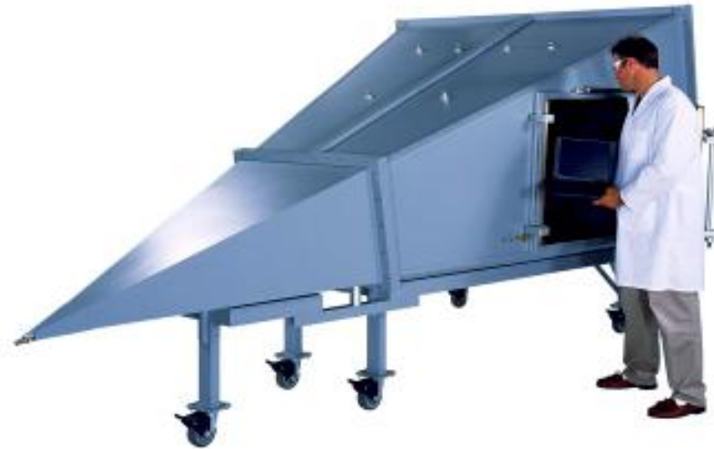
Figure 7.1 The GTEM Cell used for interference testing [69]
