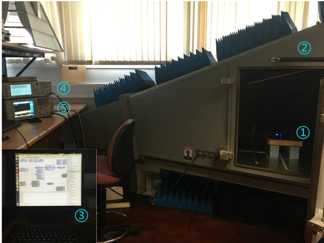
Figure 7.3 Spectrum sensing system setup in laboratory
