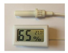
Figure 7-1 Mini portable humidity meter set
