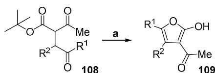
Scheme 27: Synthesis of polysubstituted furans; a: TFA or TFA/CH 2 Cl 2 (1:10). 78
