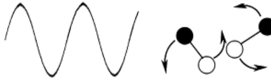
Figure 3-3: Dipolar molecules trying to align themselves according to the applied field (Lidström et al., 2001)
