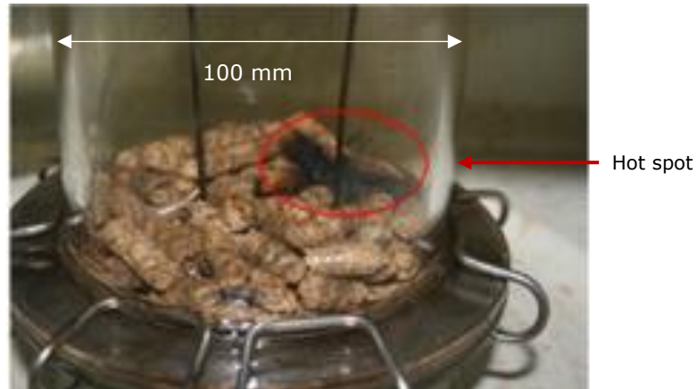
Figure 3-12: Heating heterogeneity in a multimode cavity (Salema and Afzal, 2015)
