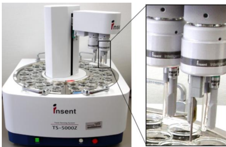
Figure 1.1: Insent Taste Sensing System TS-5000Z (Insent Intelligent Sensor Technology Inc., Atsugi-Shi, Japan). Outlined by Woertz et al. [72].
