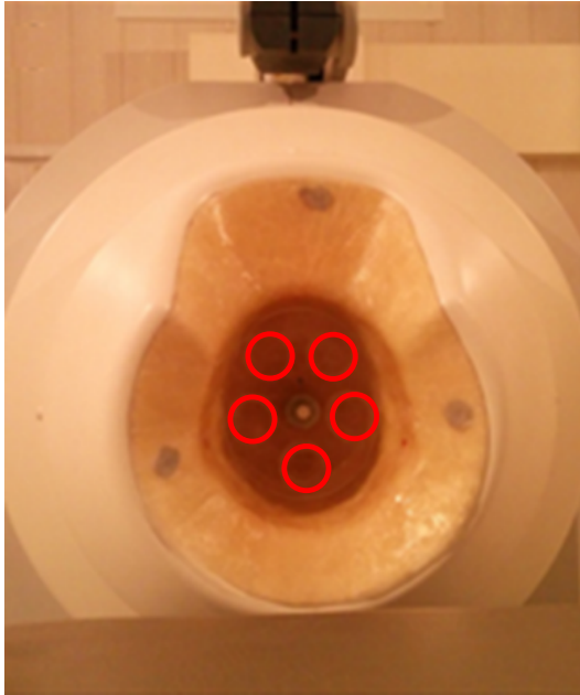
Figure 3.4: Picture of the custom-built helmet showing the location of five sample holders.
