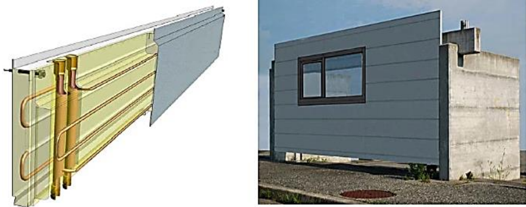
Figure 3-12 SOLABS plank hydraulic system (left) and the resulting demo site prototype (right) (Probst & Roecker, 2007)
