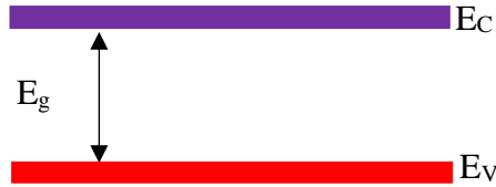
Fig. 2.4. Energy bands diagram of a semiconductor.
