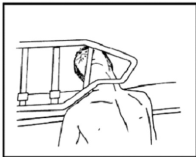
Entrapment between top of compressed mattress and bottom of rail at end of rail
