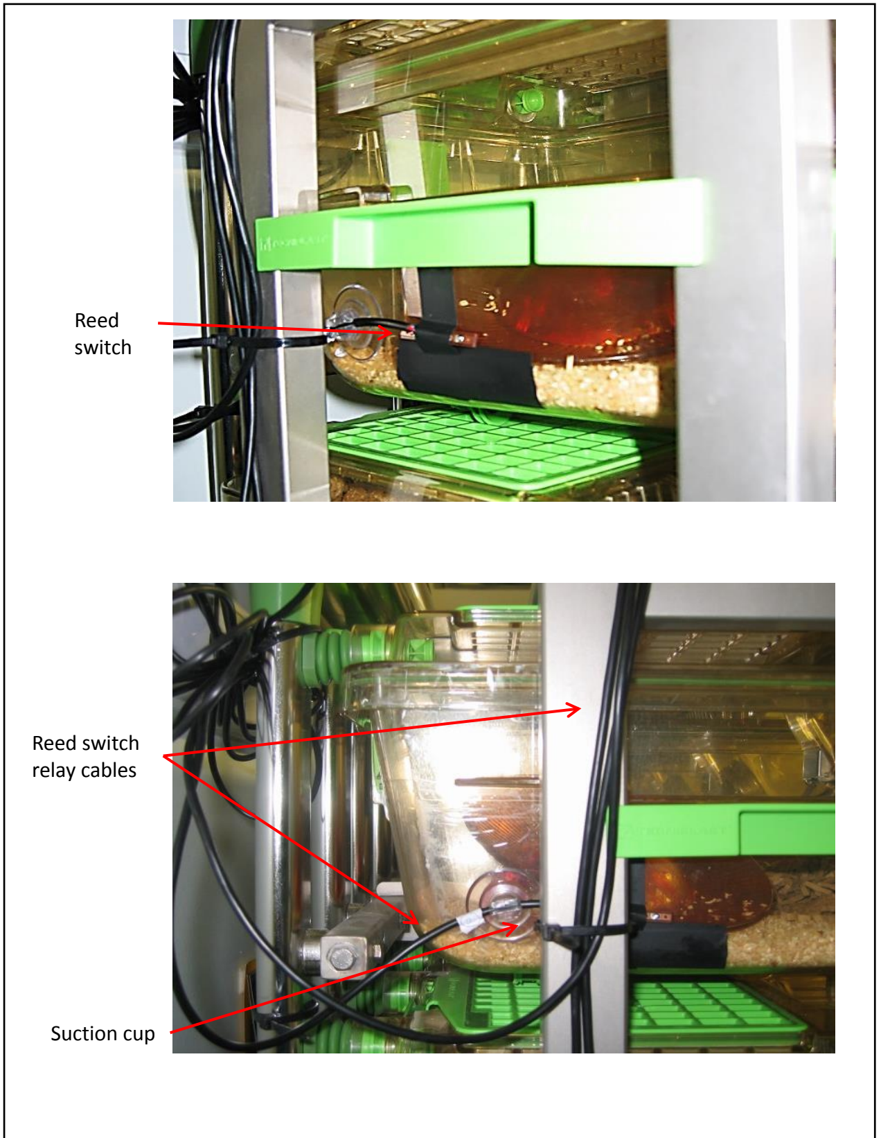
Figure 3.8 Two views of the cage docked on the rack, showing suction cup and reed switch and cables.
