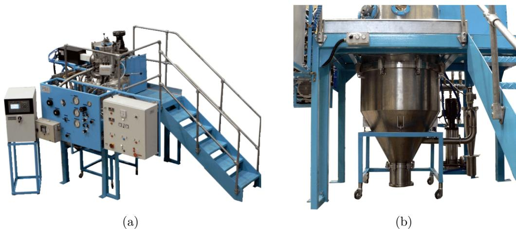
Figure 3.1: (a) PSI HERMIGA 75 atomiser with (b) hopper unit located underneath.
