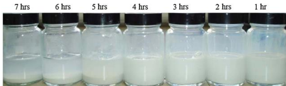
Figure 2. 5: Stability changes of \text{Al}_2\text{O}_3 nanofluid without stabilizer[29]
