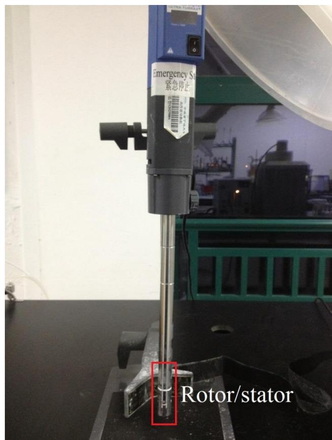
**Fig.3.4 Image of a high speed disperser (IKA T25)**
