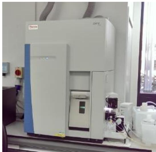
*Figure 3-28: Thermo iCAP-Q ICP-MS unit.*
