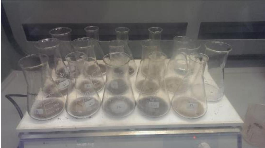
*Figure 3-26: Digestion of solid samples on hot plate.*
