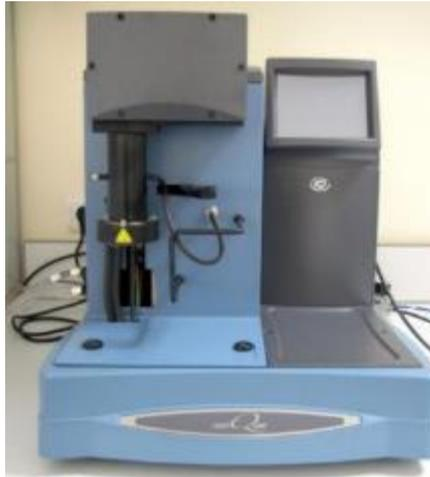
Figure 3-11: TA Instruments Q500 used for thermogravimetric analysis (TGA).
