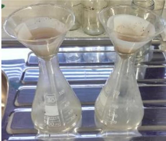
*Figure 3-9: Filtration to separate biomass from leachate.*
