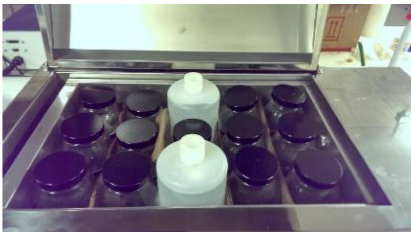
*Figure 3-8: Jars with biomass loaded, secured in the water bath.*
