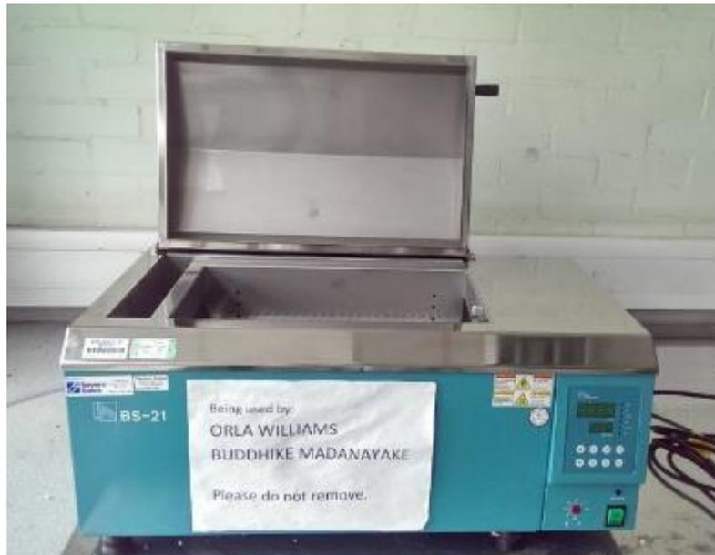
*Figure 3-6: Shaking water bath used for the leaching runs.*
