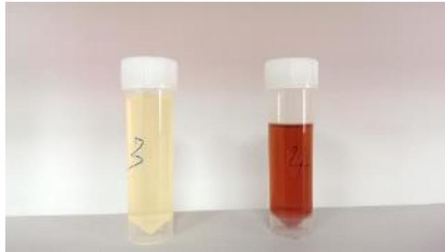
*Figure 3-27: Digested samples of (a) untorrefied, (b) torrefied biomass.*
