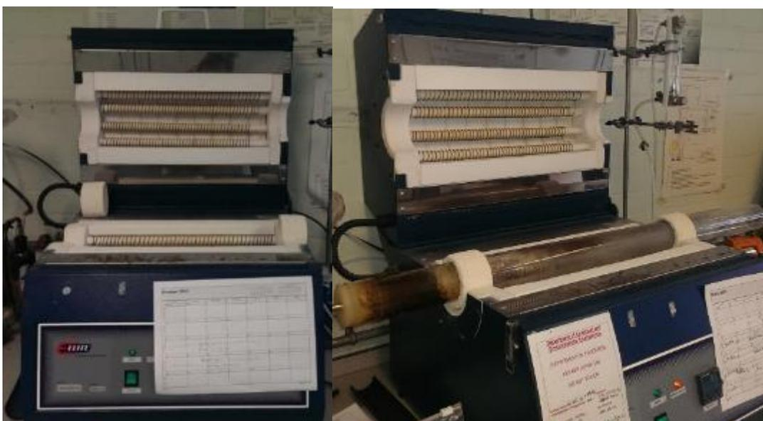
*Figure 3-4: Horizontal tube furnace used for torrefaction*
