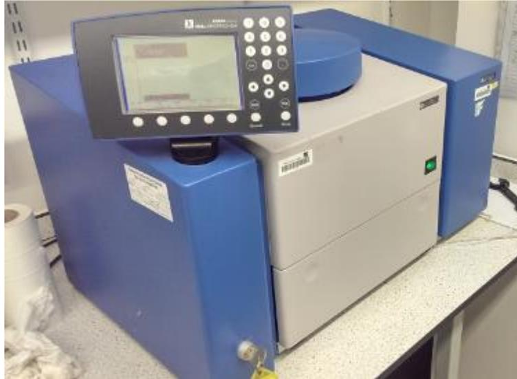
Figure 3-14: IKA C5000 bomb calorimeter.
