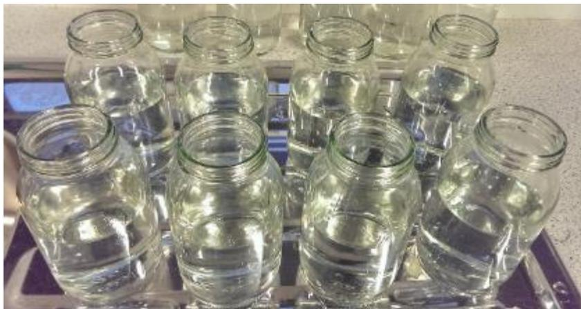
*Figure 3-7: Glass jars with Milli-Q water used for the leaching runs.*
