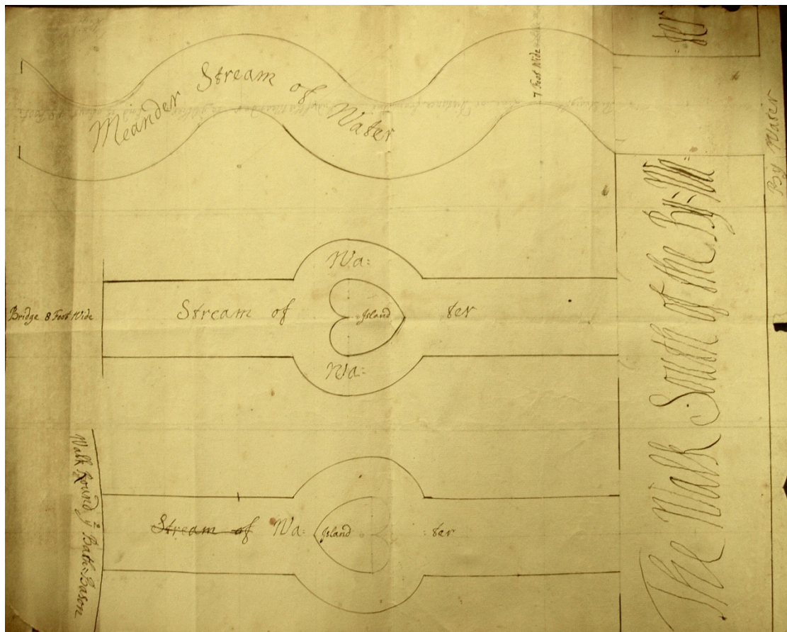
Figure 4.10: Graphic and written directions for the construction of ornamental water channels leading from the cold-bath fountain.
