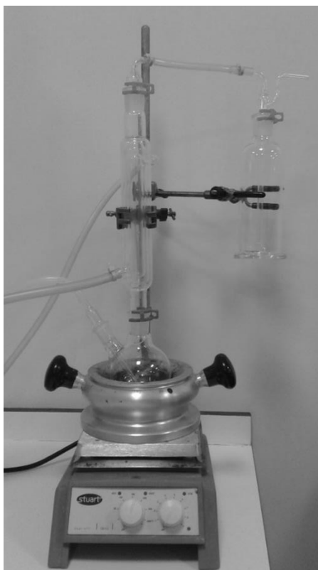
Figure 2.3: Distillation apparatus used during determination of total sulphur dioxide content
