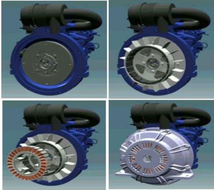
Figure 9. Possible coupling arrangement onto the engine flywheel for a permanent magnet variable speed generator [40]
