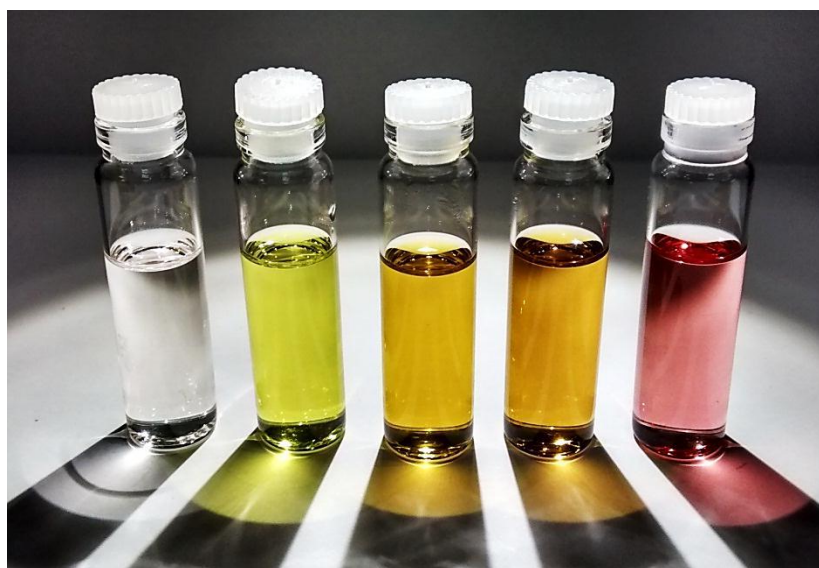
Figure 2.4: Colours of thionated NDIs as dichloromethane solutions. Left to right: NDIS 0 , NDIS 1 , NDIS 2 cis, NDIS 2 trans and NDIS 3 .
