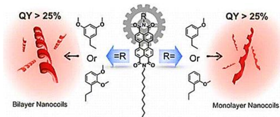
Figure 4.1: Schematic depicting the self-assembly of asymmetric PDIs into fluorescent mono- or bi-layered nanocoils by control of a methoxyaryl imide group. Adapted from Liu et al. 19
