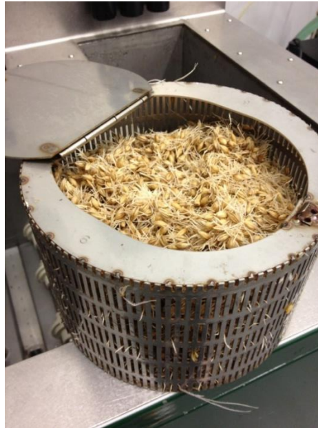
Figure 26. Steep/germinator cylindrical vessel used in the research containing germinated barley.
