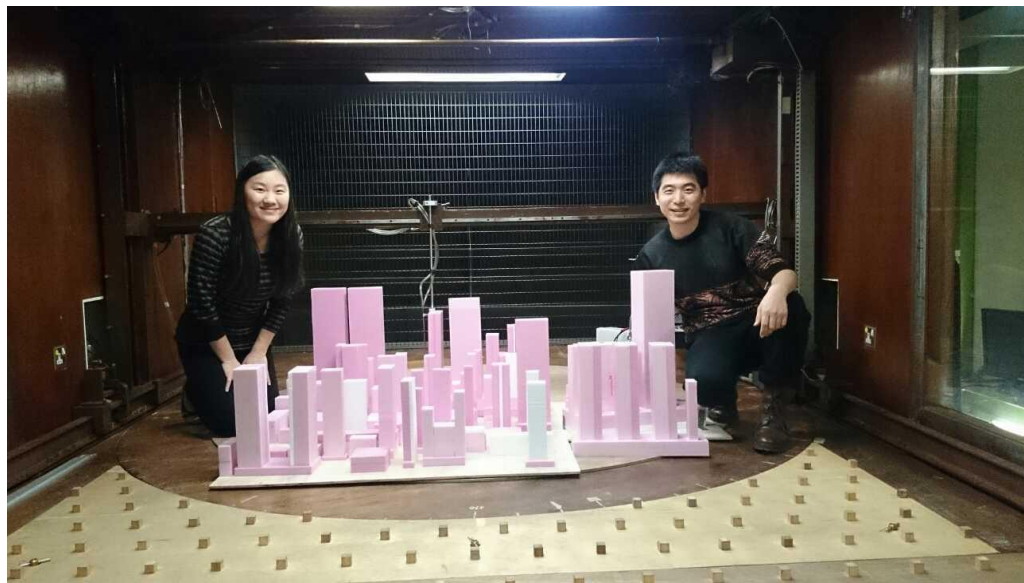
Figure 15: Test case of high-rise building models in wind tunnel
