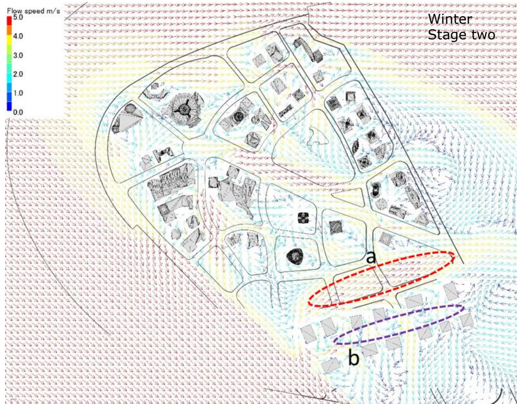
Figure 62: Outdoor pedestrian-level wind environment (Order B)
