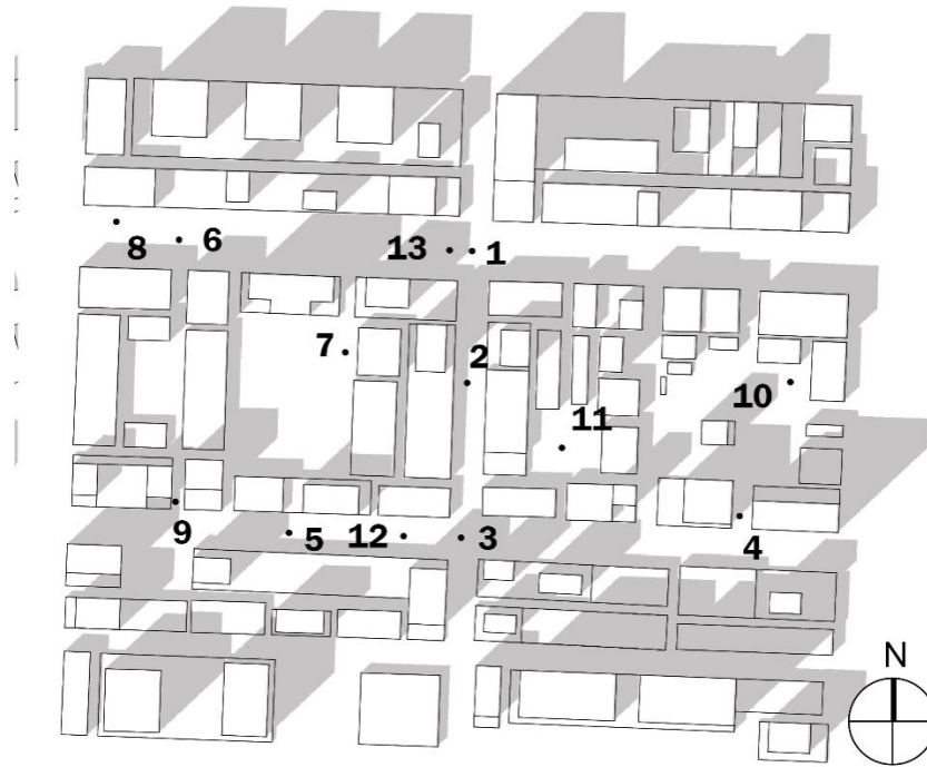
Figure 21: Positions in the site for comparing the results of wind tunnel tests and numerical simulation
