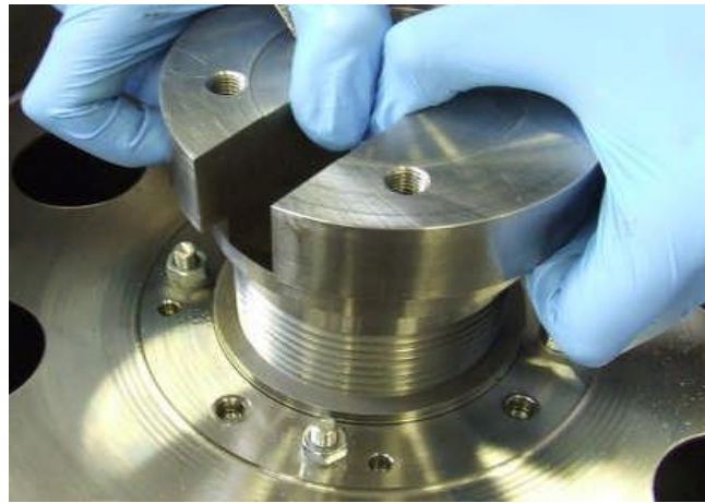
Figure 4.9 Installation of the Labyrinth Seal Plug
