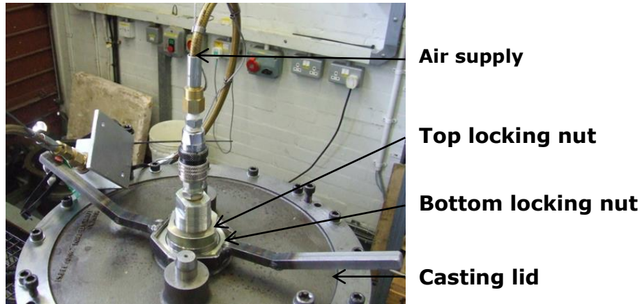
Figure 4.4: Fixation of seal assembly with the top casting lid
