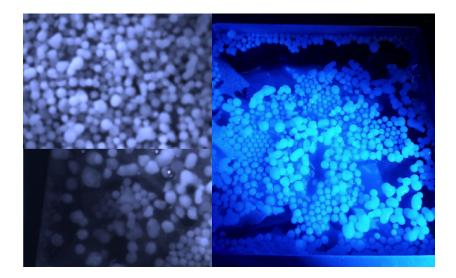
Figure 2: Ice granules in a closed glass cassette vibrated by an electromagnetic shaker, in a temperature controlled chamber at -3°C. Top left: A dry granular gas, after 5 minutes of shaking. Bottom left: After 20 minutes of shaking, larger coalesced particles appear alongside pockets of close packed particles. Right: Once all of the granules stopped moving after 65 minutes of shaking, the cassette was opened.
