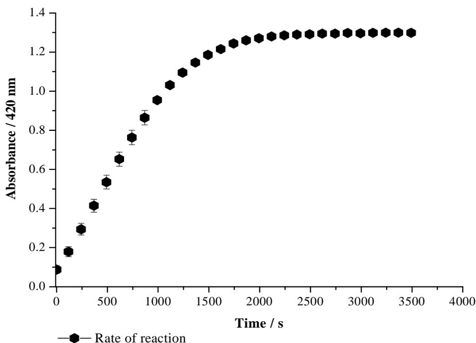
**Figure 3.1:** The time course of ABTS oxidation by LTV.
