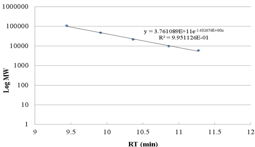
**Figure 2.8:** GPC calibration curve using pullulan standards
