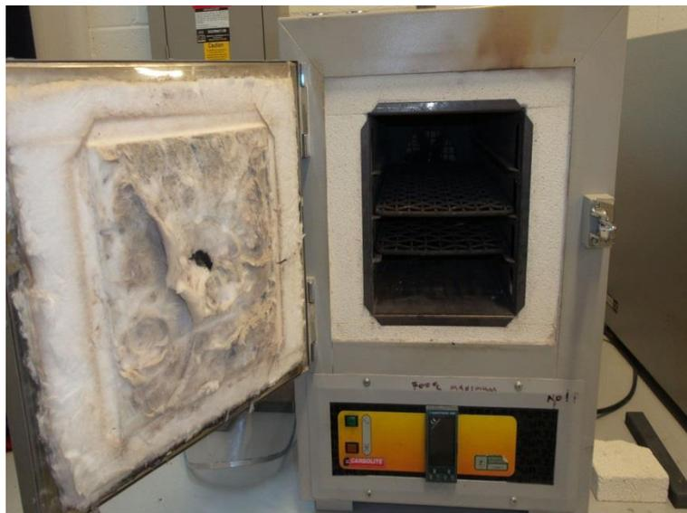
Figure 3.7 Oven for heat treatment
