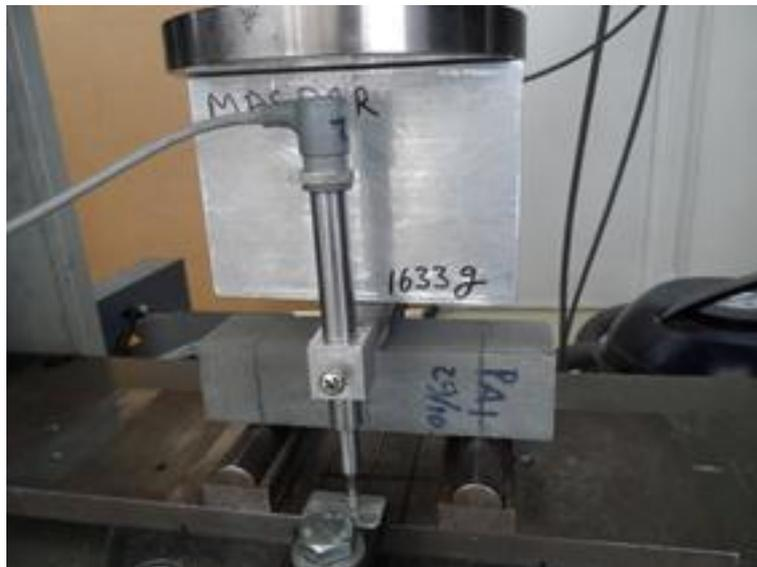
Figure 3.11 Setting up the LVDT on two sides of a prism
