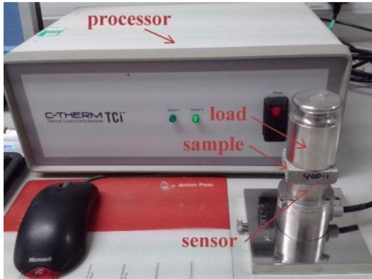
Figure 3.13 Setting up thermal conductivity test
