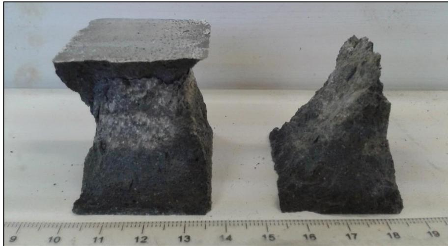
Figure 4.5 Normal failure mode of RPC in compression forming a double pyramid shape
