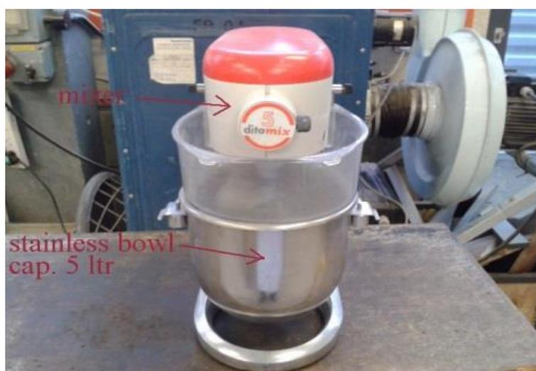
Figure 3.4 Small concrete mixer with adjustable speed setting.
