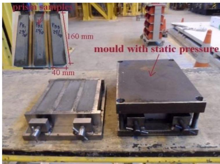
Figure 3.5 Mould with and without pressure
