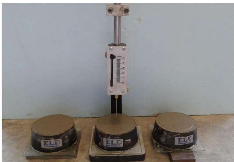
Figure 3.8 Setting time apparatus
