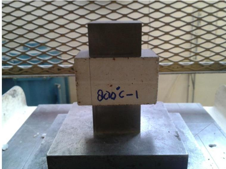
Figure 3.12 Setting out of sample for compressive test
