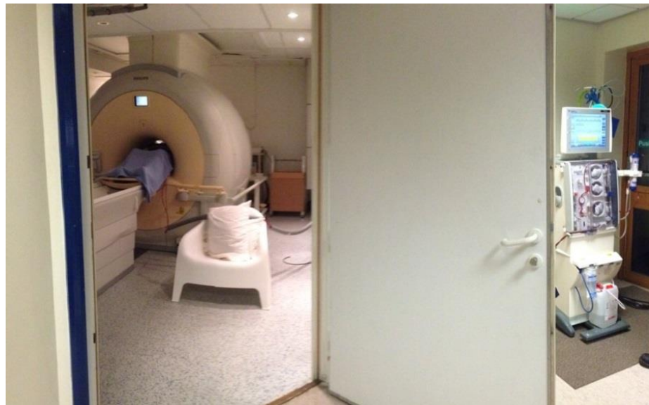
Figure 4.2-1: Photo of the setup showing the dialysis machine outside of the MR scan room and the patient inside the scanner. To the left of the scanner, the extension lines with insulation can be seen.
