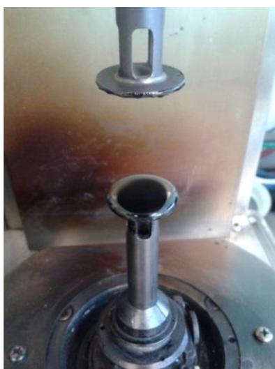
**Figure 4-1: Image of PIBSI 65% MicroCB 35% sample on rheometer plate prior to analysis.**
