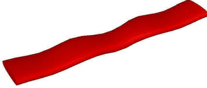
Figure 3.15 Model of the yarn with curved path and variable cross-section
