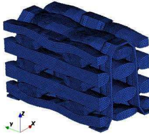
(b) Yarn mesh generated by HyperMesh (only those for the yarns are shown)
