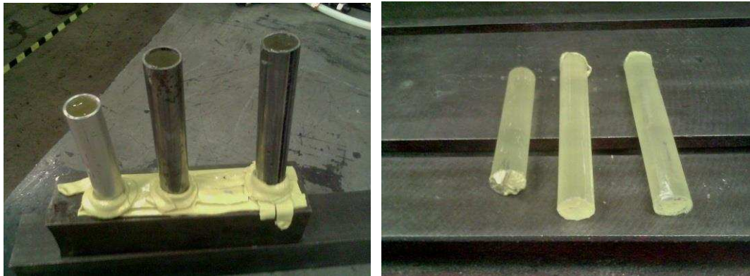
(a) Aluminium tubes filled with the resin (b) Cured resin samples
