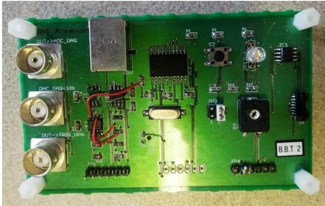
Figure 3.17 - Assembled second ECG processor board
