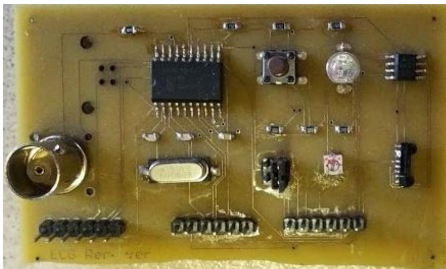
Figure 3.6 - First ECG processor assembled
