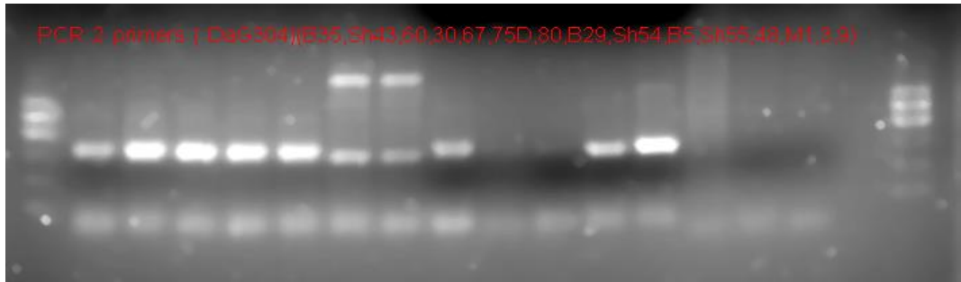
Figure 4.50 PCR, static Ta 50 0 C for D. alata , D. bulbifera , and D. cayenensis species incorporating Da3G04-350bp primers. The positive results were observed on 1% agarose gel.
