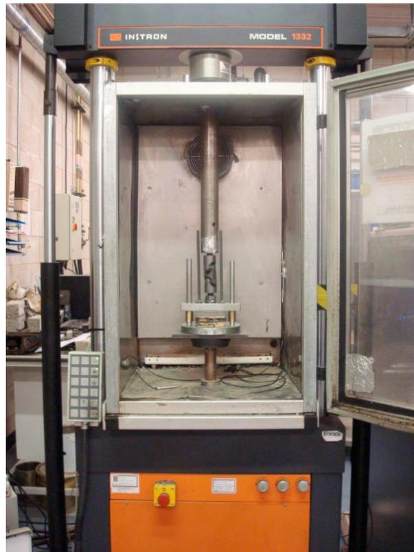
Figure 2-12 Test equipment for pull-off test using UTM [75]
