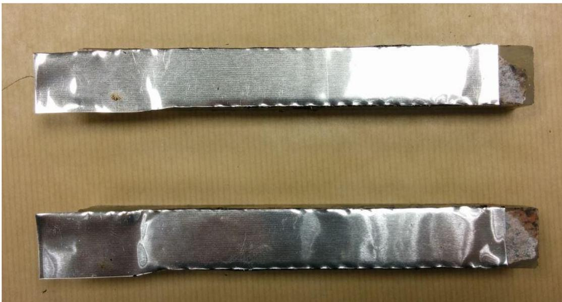
Figure 7-4 Prepared adhesion specimens used for peel test
