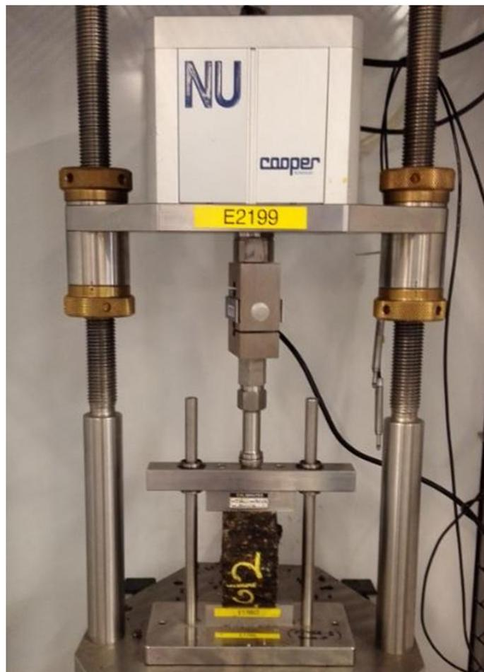
Figure 2-5 Test equipment for determination of indirect tensile strength or stiffness
