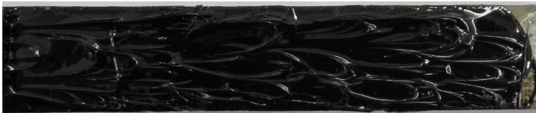
Figure 7-8 Failure surface of specimens prepared with G2 coarse aggregates in dry condition
