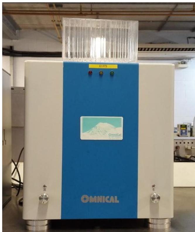
Figure 2-10 Image of the Microcalorimeter equipment
