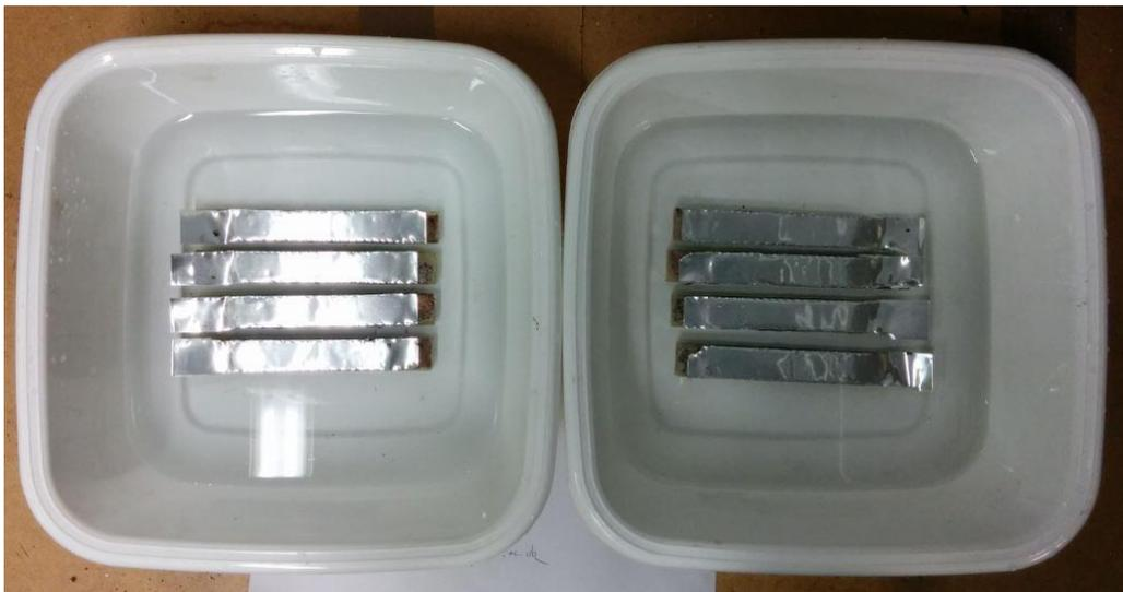
Figure 7-5 Moisture conditioning of adhesion specimens
