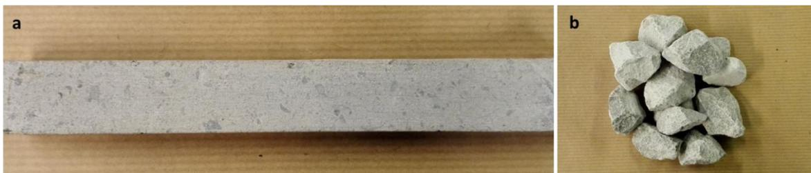
Figure 7-1 Aggregate substrate and coarse aggregates: (a) substrate must be prepared from large boulders, while (b) coarse aggregates are readily available in most labs.
