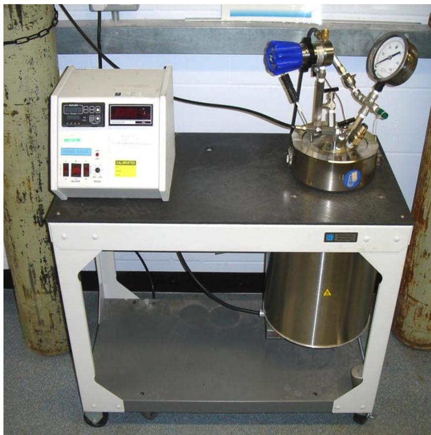
Figure 2-14 Equipment used for the SATS test
