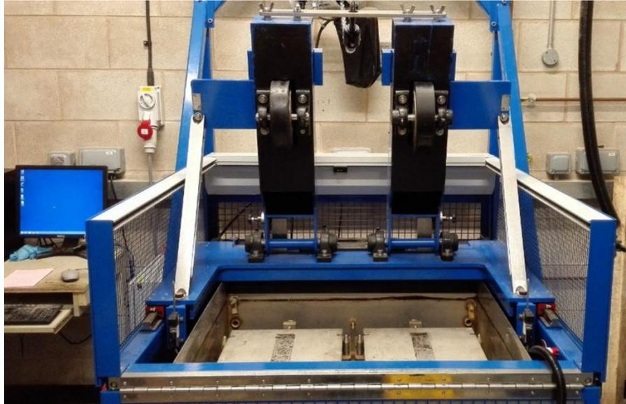
Figure 2-6 Hamburg wheel tracking device for determination of permanent deformation
