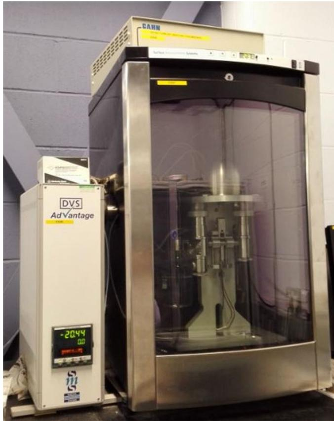
Figure 2-9 Image of the Dynamic Vapour Sorption equipment
