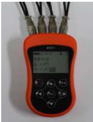
Figure 5-4: WT0T1-9-02 Temperature data logger
