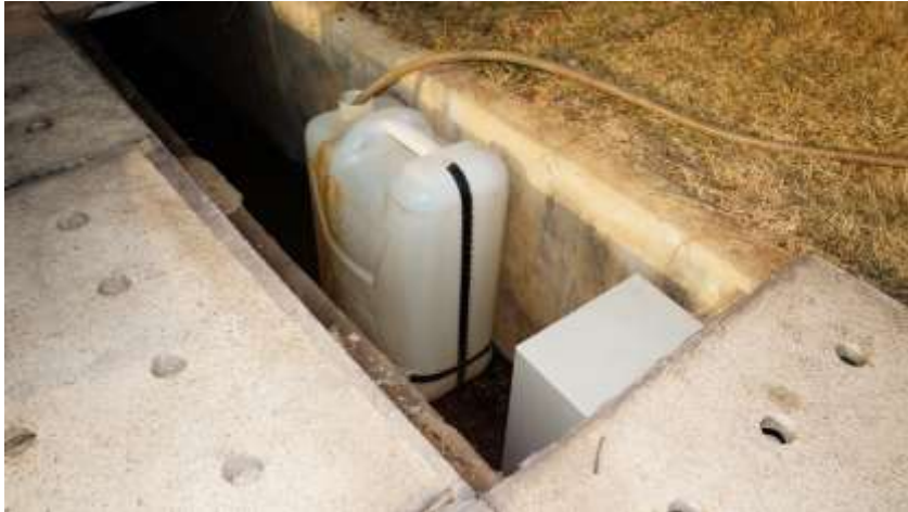
Figure 5-13: Drain measurement setup- graduated semi clear container
