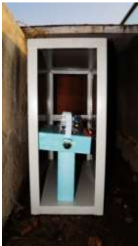
Figure 5-14: Drain measurement setup- Raspberry-pi/camera assembly placed facing the container
