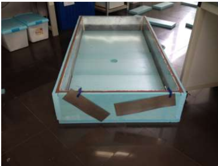
Figure 5-1: Test cell under construction-XPS boards are being attached to the stainless steel box
