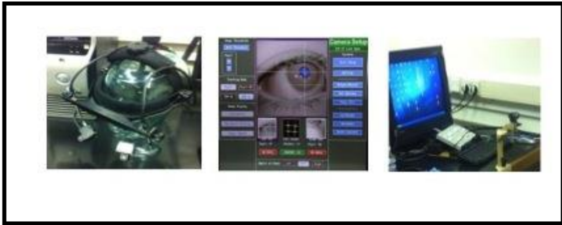
Figure 2.1. Illustration of EyeLink equipment: Binocular head-mounted with Camera Setup Screen and Display Computer.
