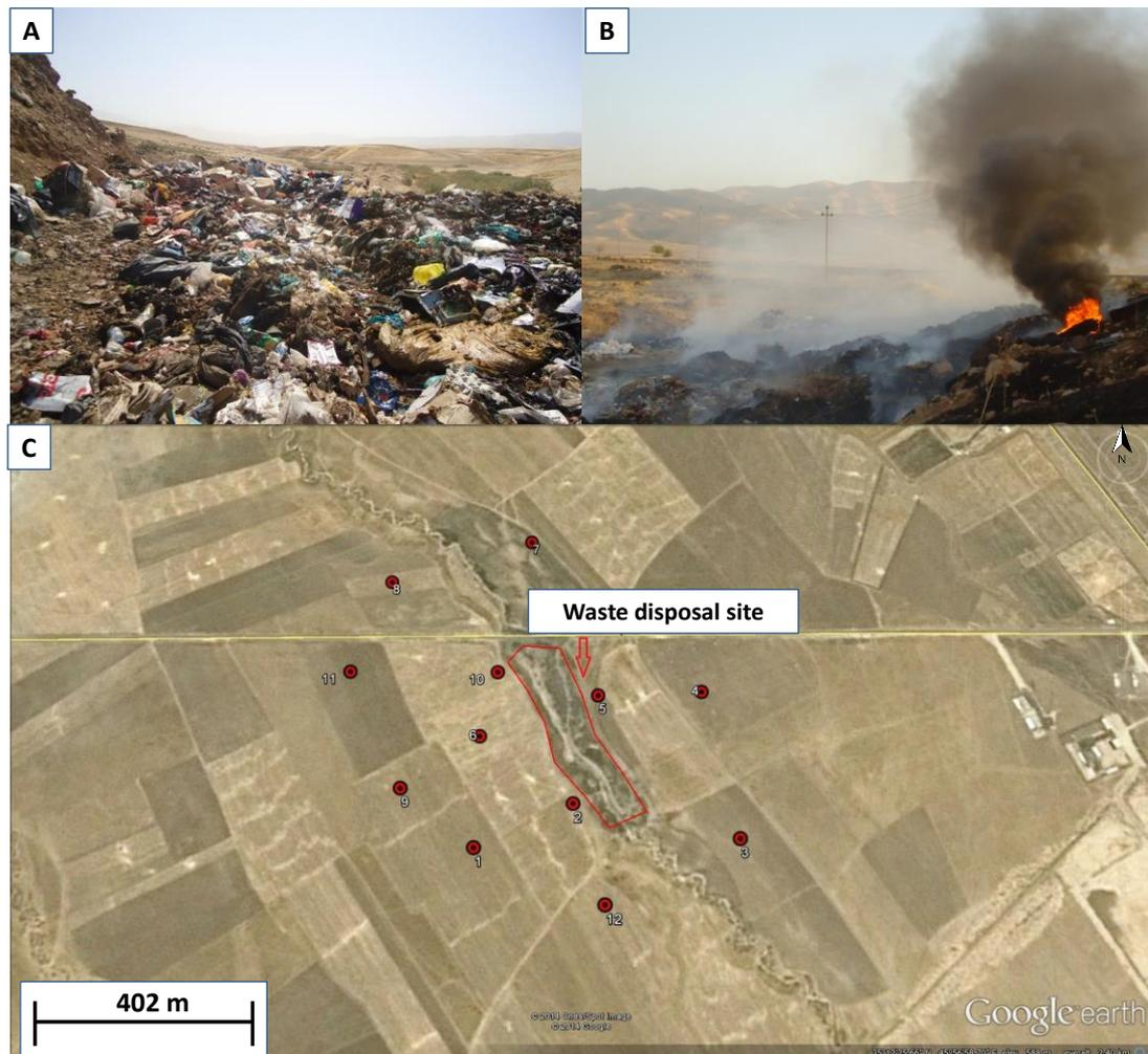
**Figure 3.4** Halabja solid waste disposal site (a) where incineration of waste (b) is common. Satellite image of disposal area (c) surrounded by agricultural land showing soil sampling sites (red).
