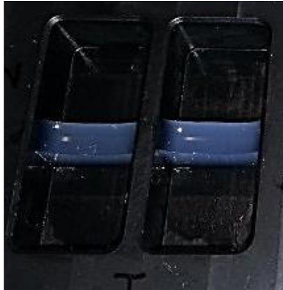
**Figure 14: Top view of compartmentalized diffusion chamber showing hydrogel membranes of  $15 \times 5 \times 6.6$  mm (Length  $\times$  Width  $\times$  Height) dimensions cast in the middle of the chamber.**
