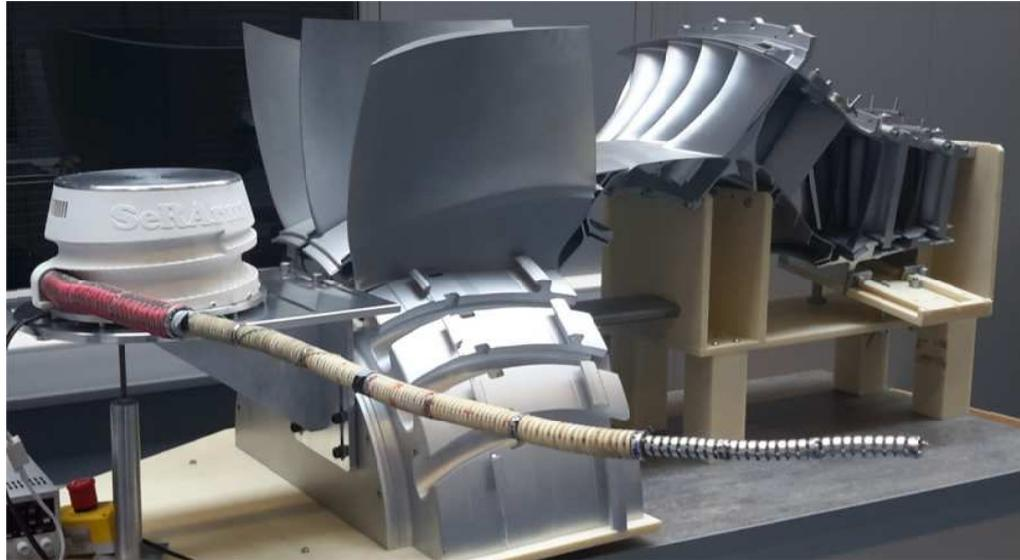
Figure 6-21. the assembly of the final full length continuum robot
